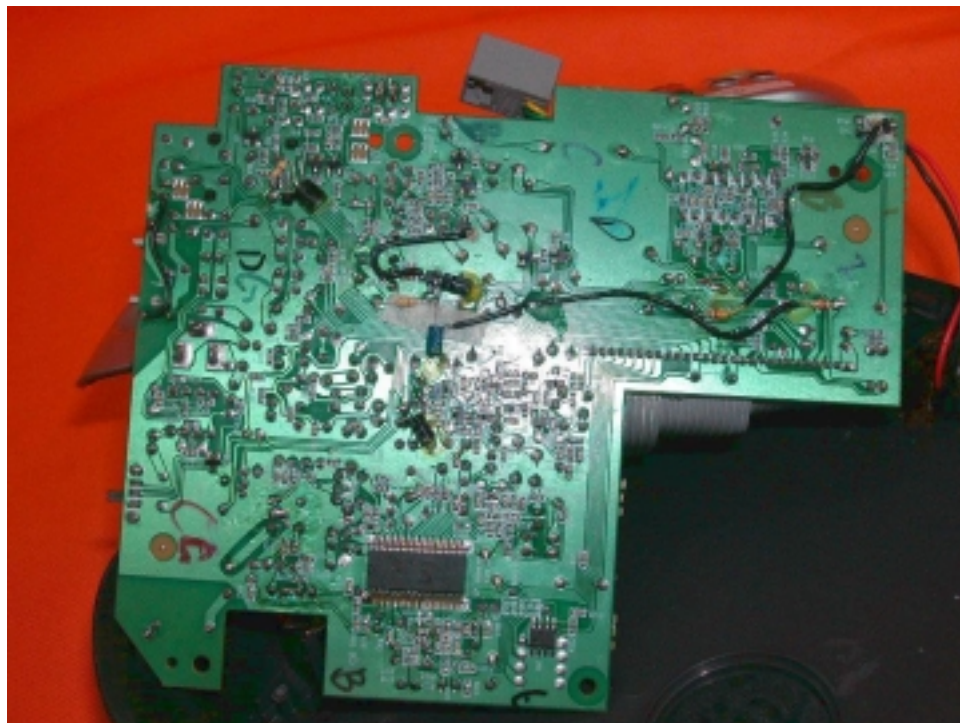
Base Main PCB solder side
