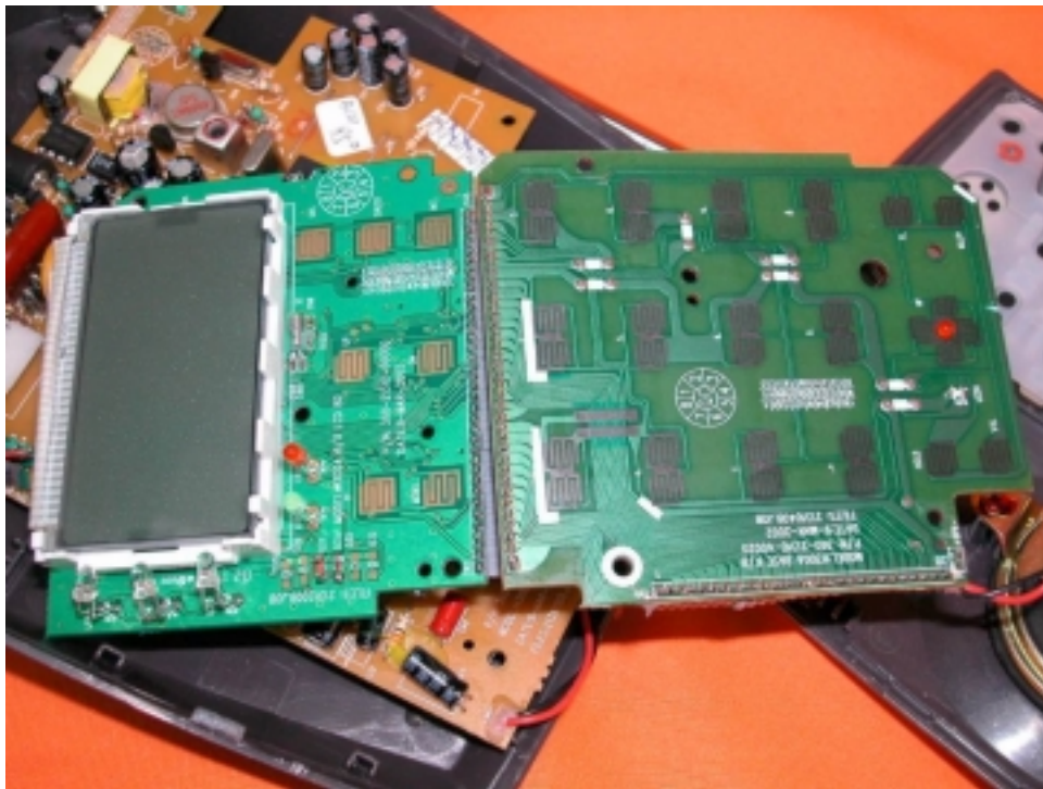
Base PCB display and keypad side
