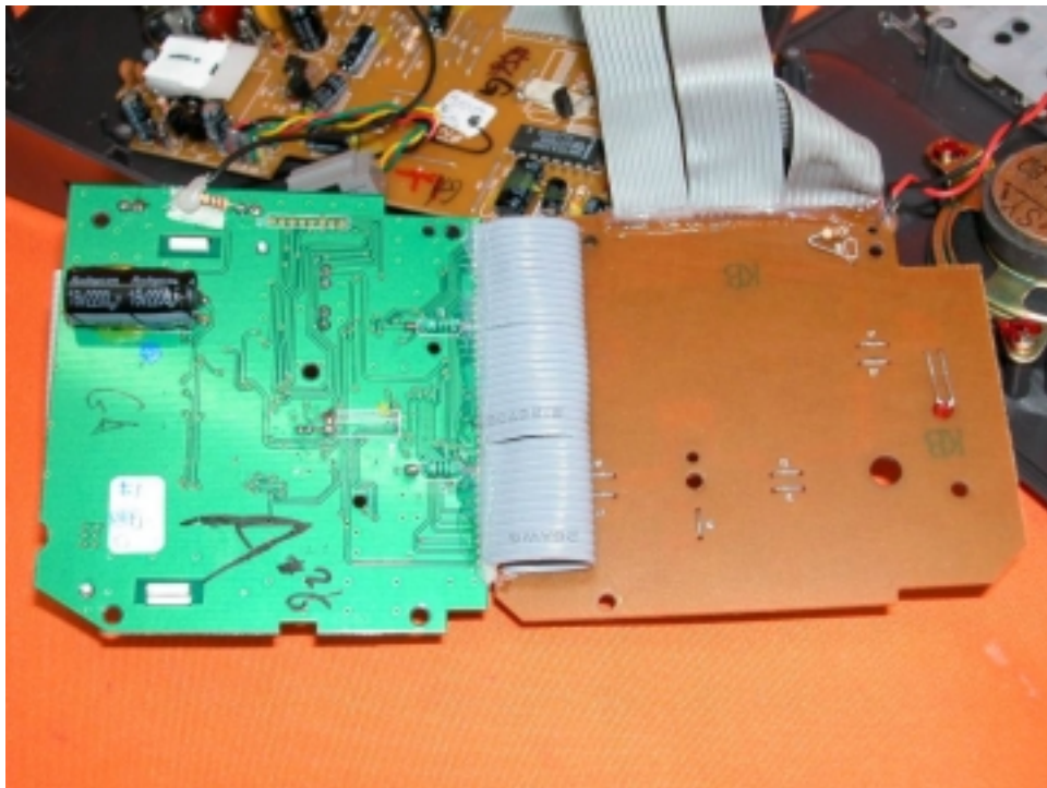
Base PCB display and keypad rear side
