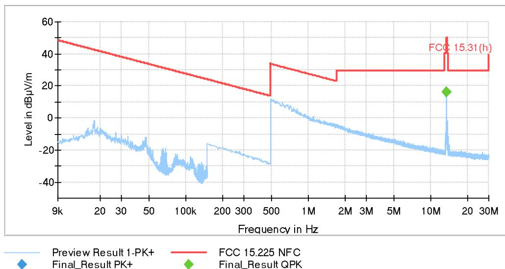
The highest peak is the RFID 13.56 MHz carrier frequency.
