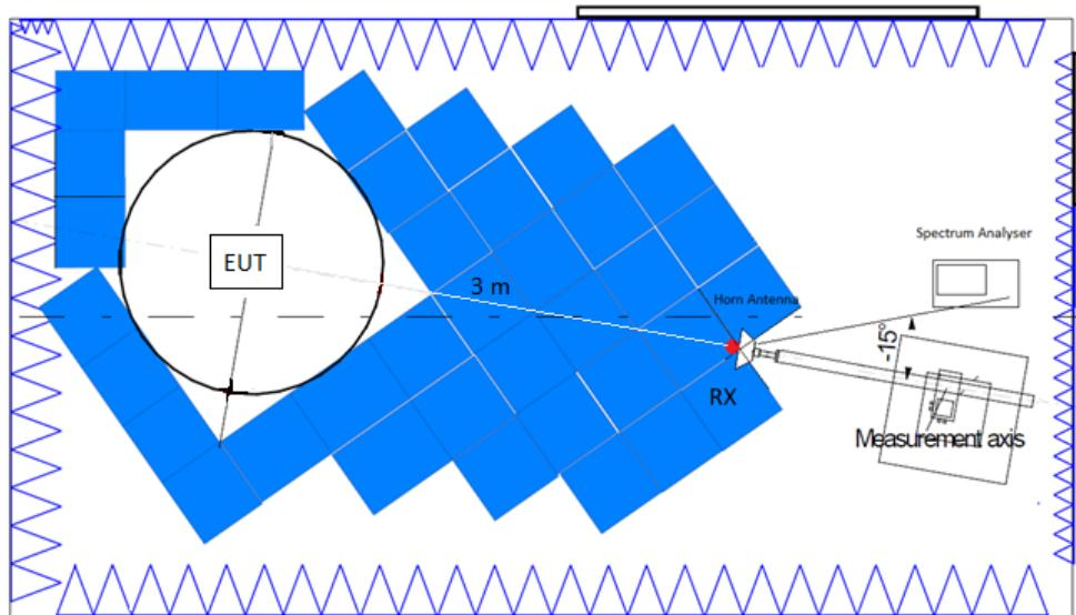
Radiated measurements setup  $f > 17$  GHz:
