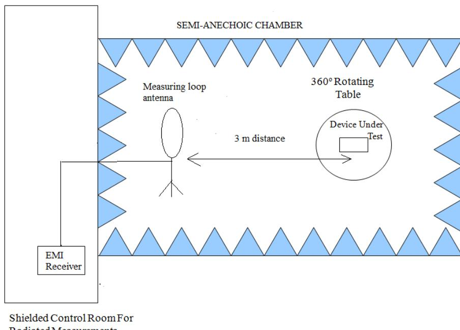
Radiated measurements setup  $30 \text{ MHz} < f < 1 \text{ GHz}$ :
