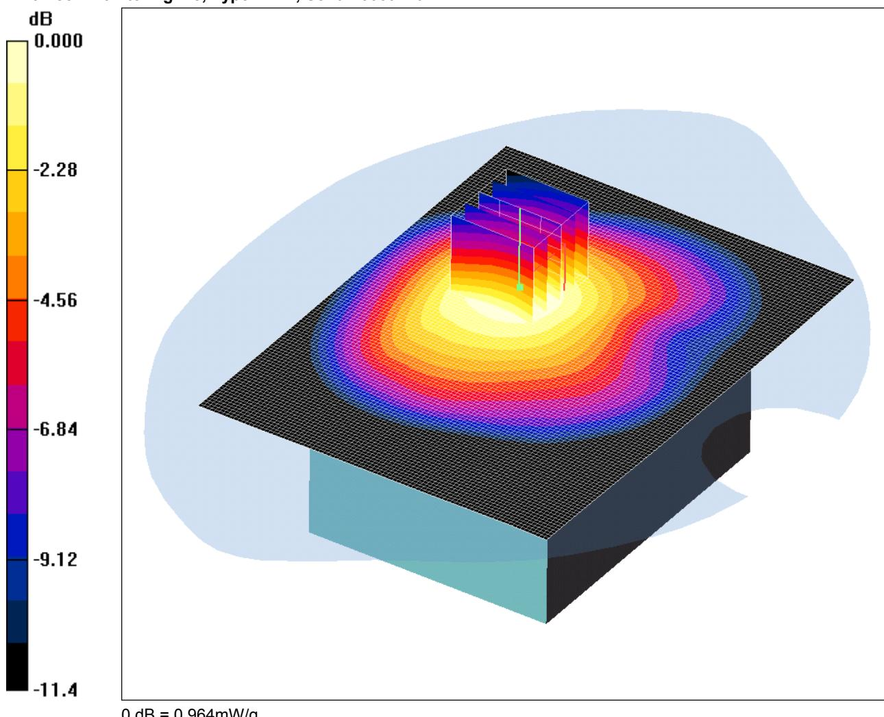
Communication System: 850 MHz; Frequency: 848.8 MHz; Duty Cycle: 1:8.3
