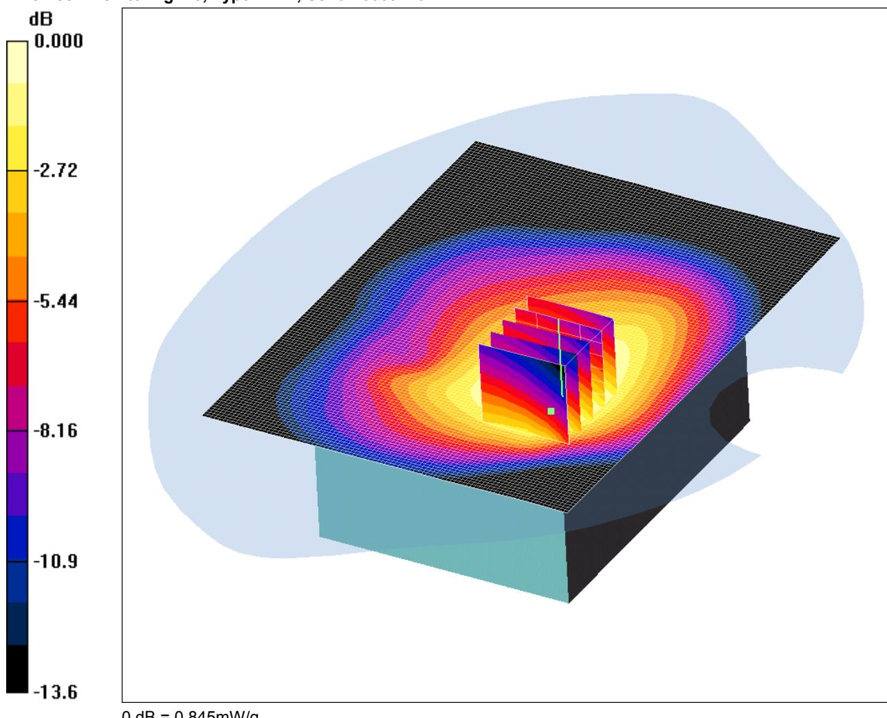
Communication System: GPRS 850 MHz; Frequency: 824.2 MHz; Duty Cycle: 1:4
