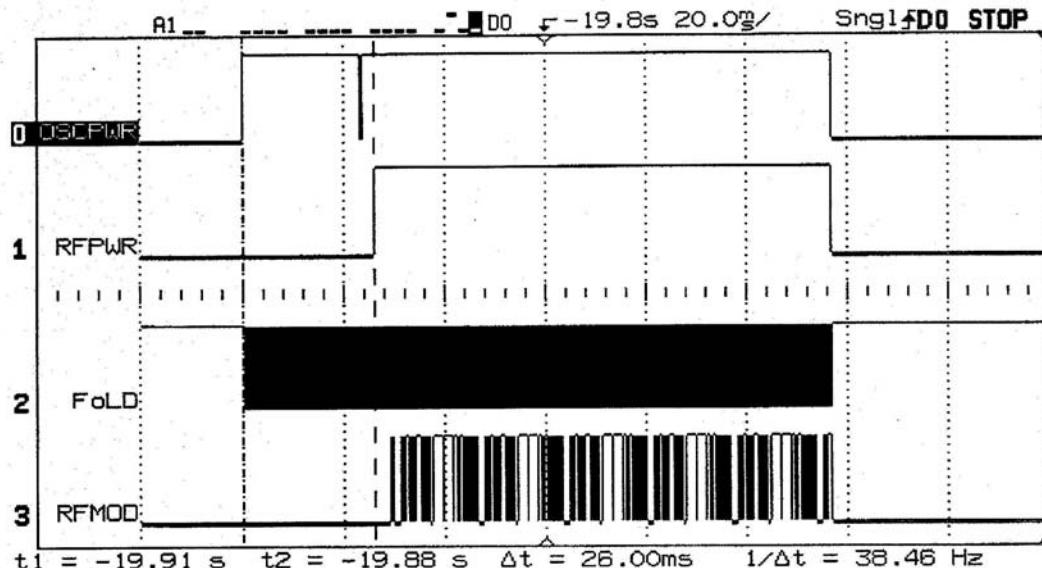
The duration of the transmission is less than one second and the silent time is greater than 10 seconds.
