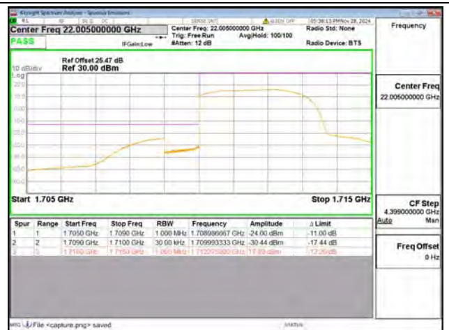
B66 / 3MHz / Low CH / QPSK / FULL RB
