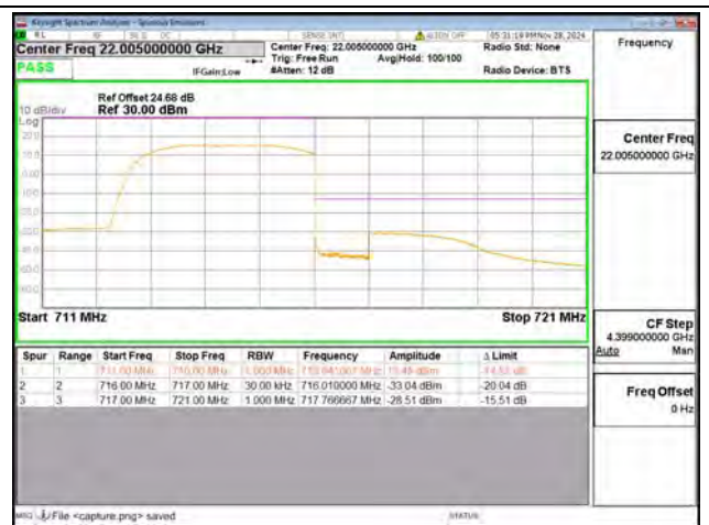
B12 / 3MHz / High CH / QPSK / FULL RB
