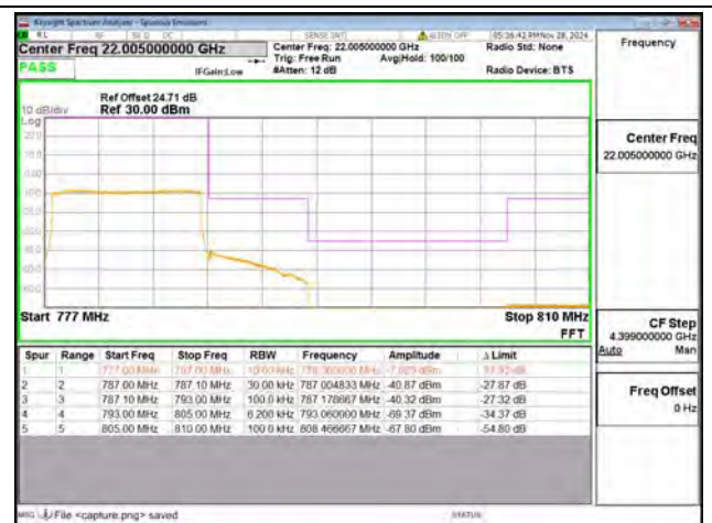
B13 / 10MHz / High CH / QPSK / FULL RB
