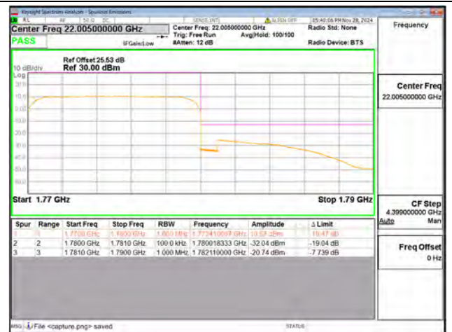
B66 / 10MHz / High CH / QPSK / FULL RB
