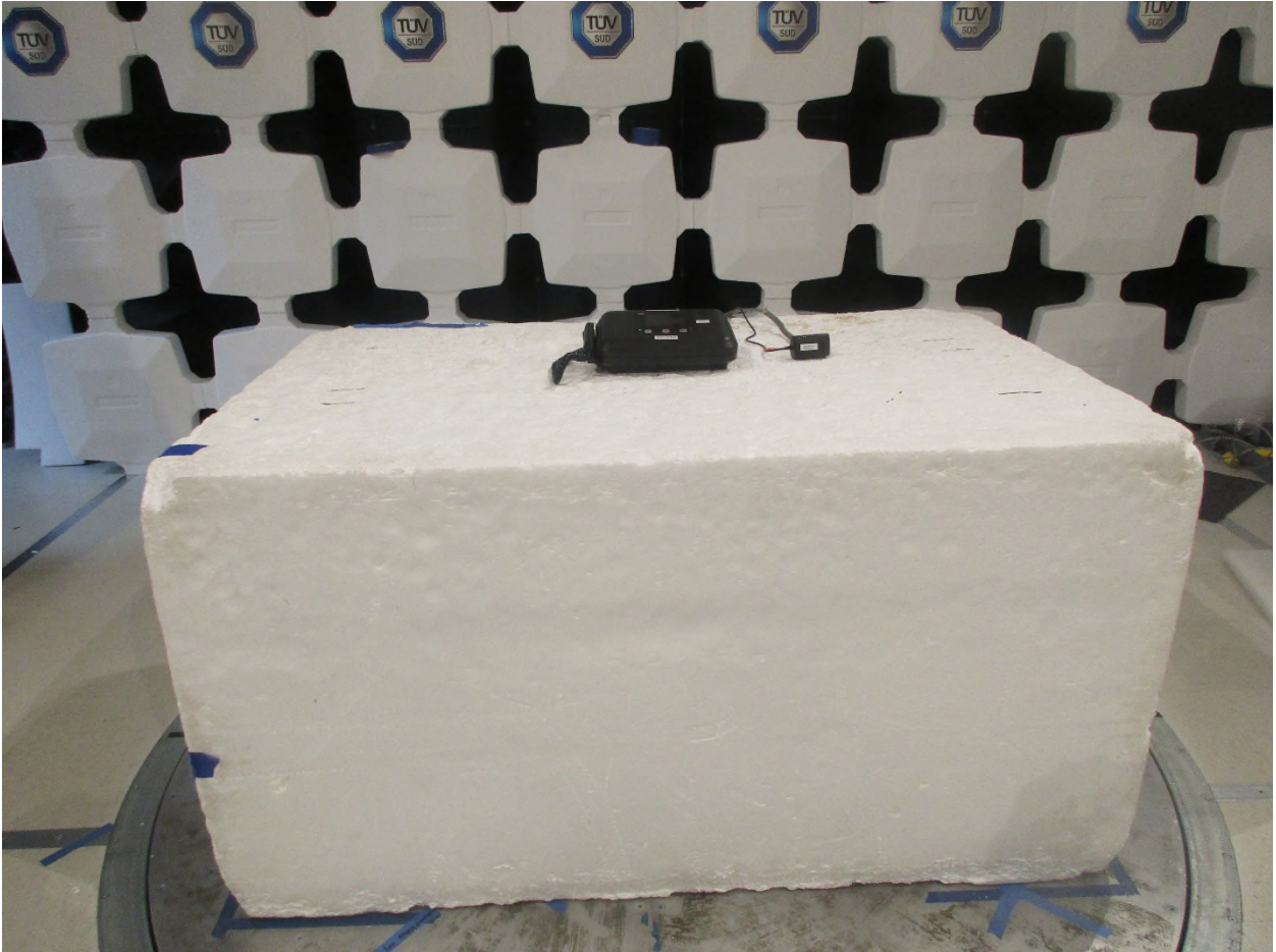
Figure 1: Radiated Spurious Emissions – Front View – below 1 GHz
