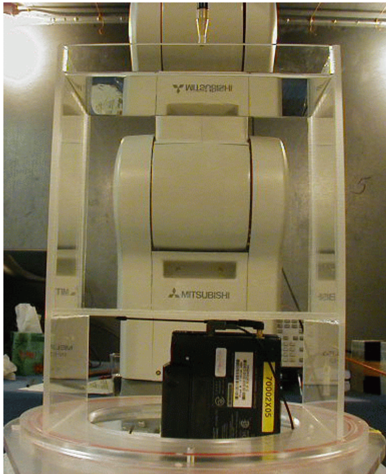
Figure 14. Position #1 - Antenna vertical and parallel to the phantom - PCS 1900 MHz
