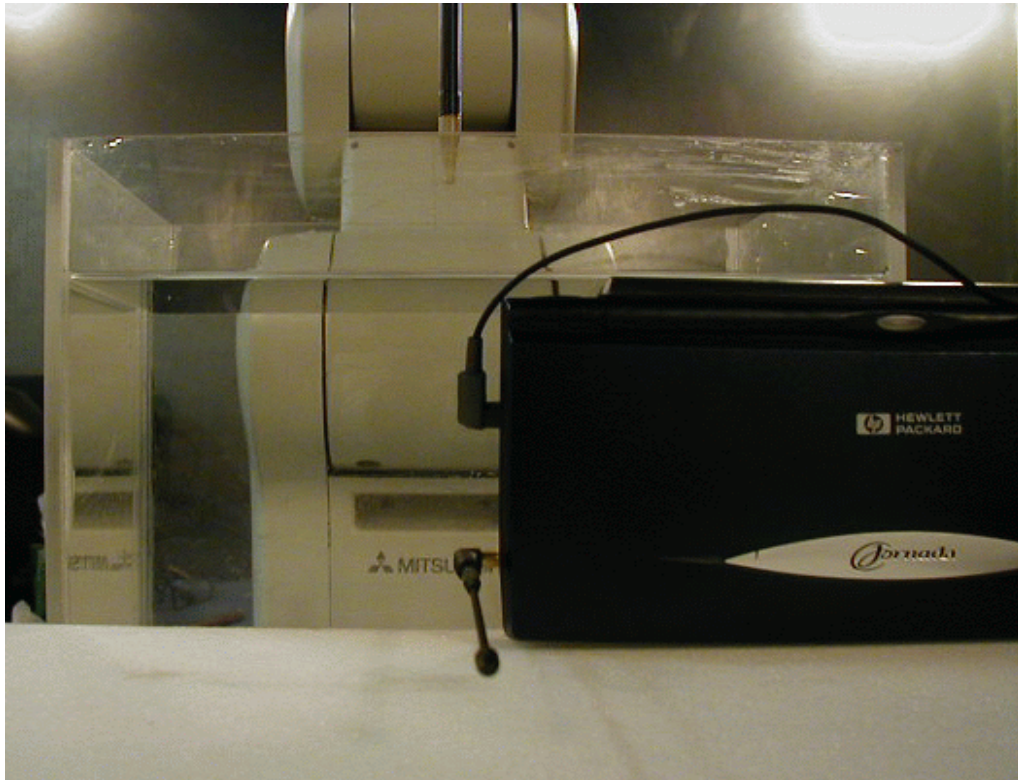
Figure 19. Position #6 - Antenna perpendicular to the phantom with headset - PCS 1900 MHz
