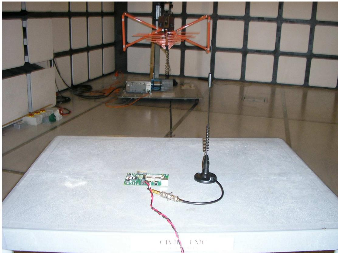
Test Set-Up Novatel Wireless EU740
