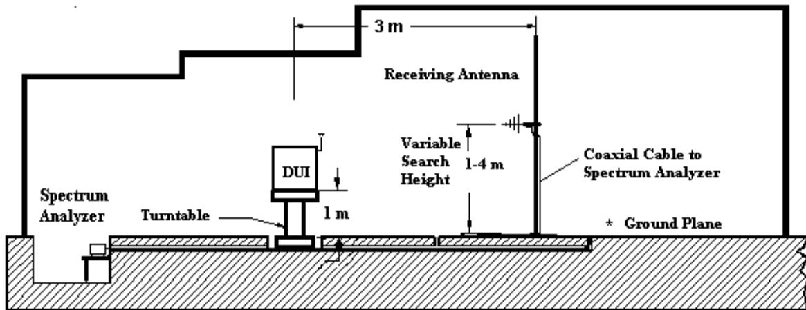
Figure 1.a Test set up for the Field Strength of Spurious Radiation Measurement in OATS
