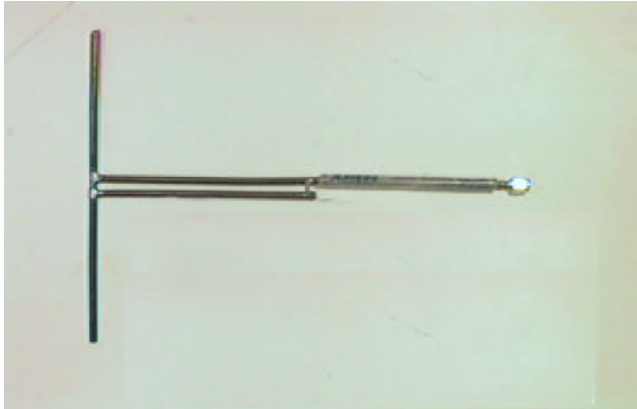
Reference Dipole Antenna Used for ERP Measurement
