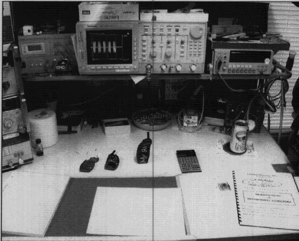
Photo 14: Oscilloscope Measurement of Raw RF timing
