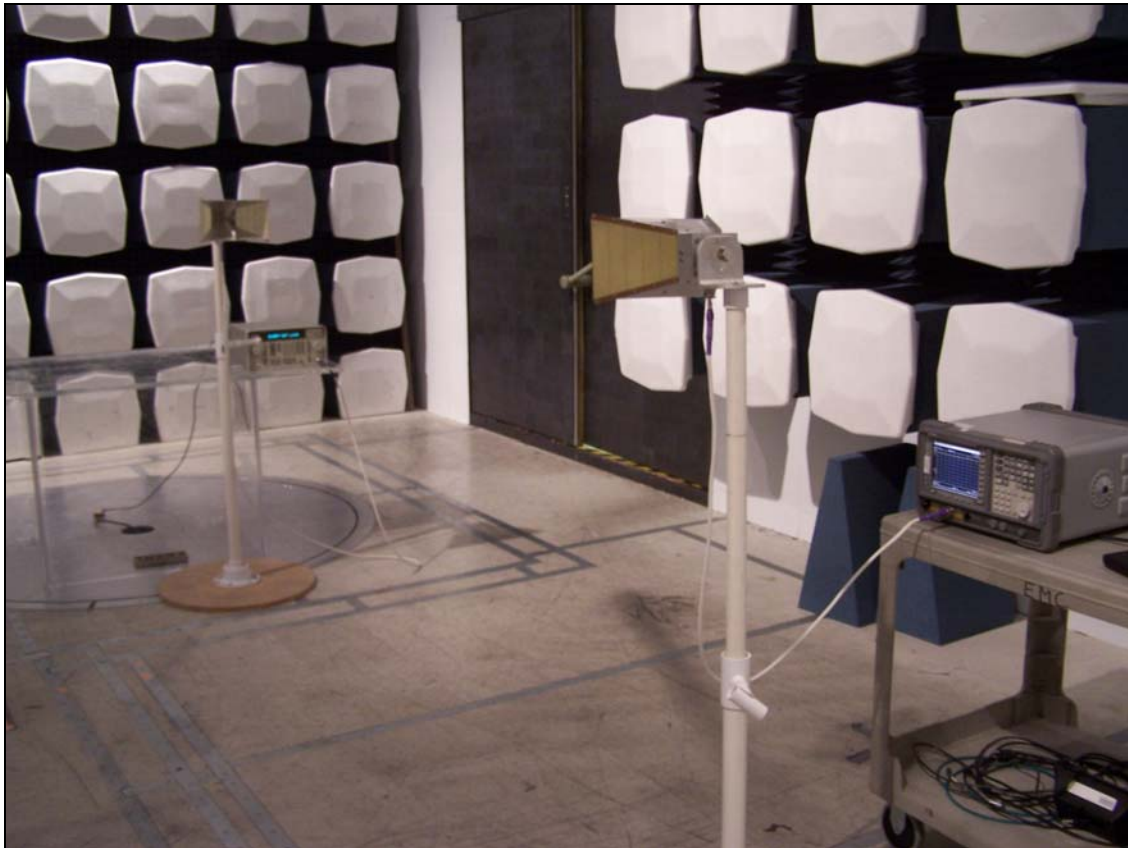
Photograph 3. Spurious Emissions Test Setup
