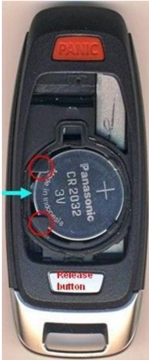
Picture 7: FS197R, rear cover removed
