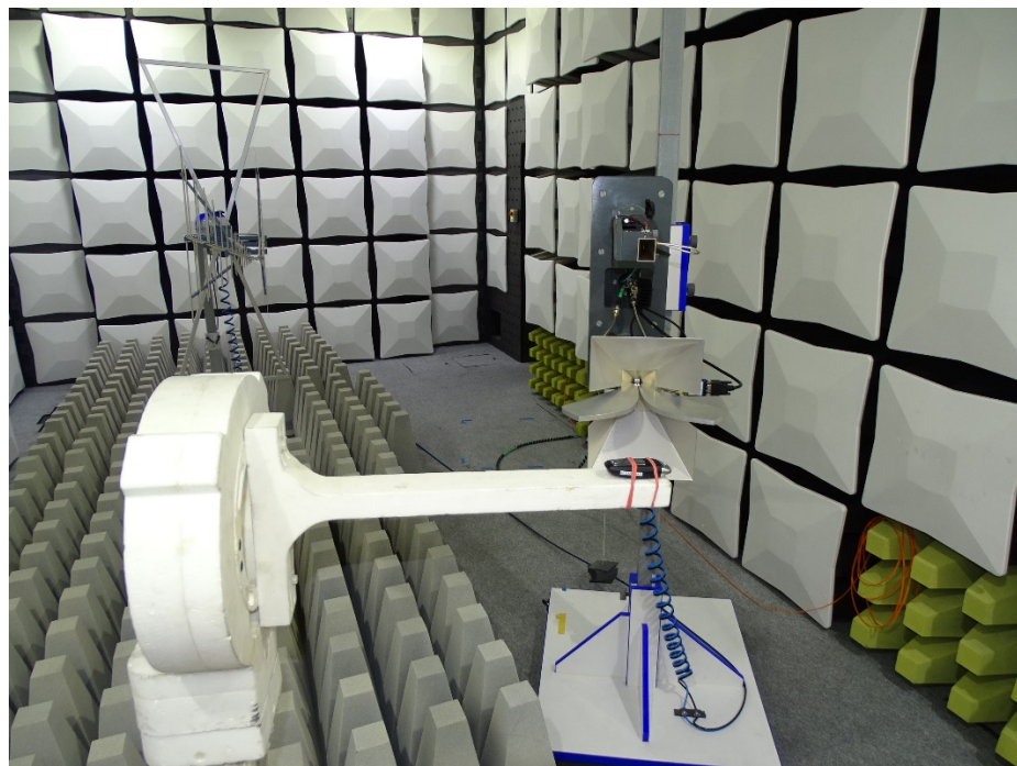
Photo 4: Test setup for radiated emissions measurements in fully-anechoic chamber (18 GHz to 26.5 GHz), rear side view, 0.5 m measurement distance
