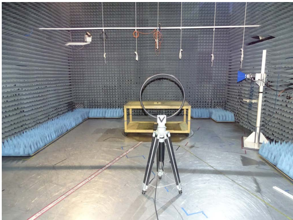
Photo 1: Test setup for radiated emissions measurements in semi-anechoic chamber (9 kHz to 30 MHz), rear side view, 3 m measurement distance
