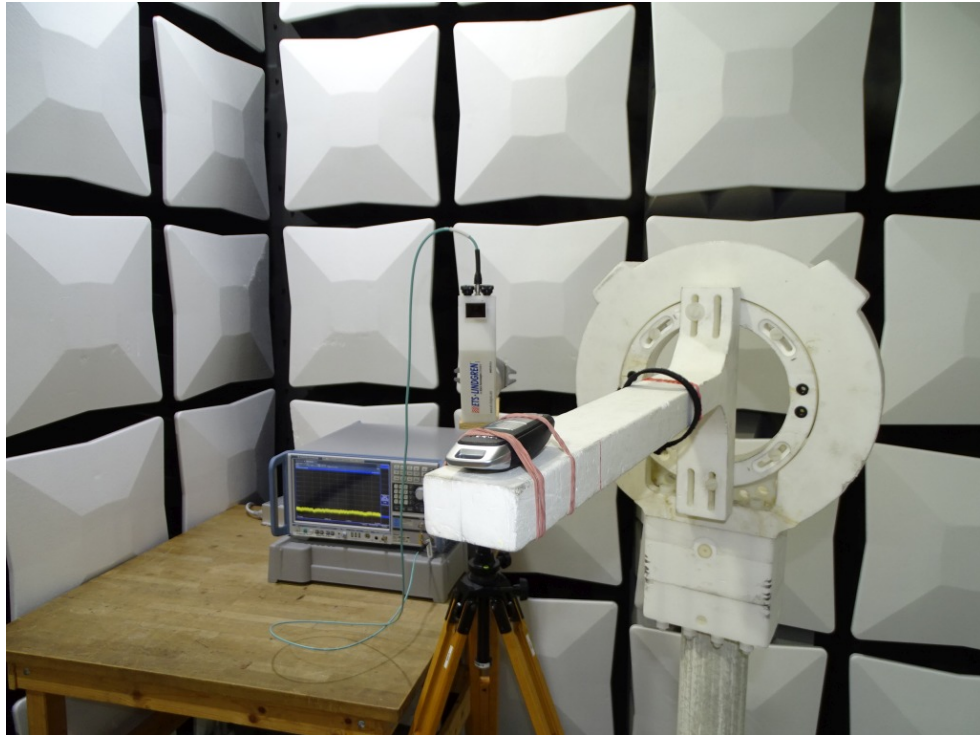
Photo 5: Test setup for radiated emissions measurements in fully-anechoic chamber (26.5 GHz to 40 GHz), rear side view, 1 m measurement distance
