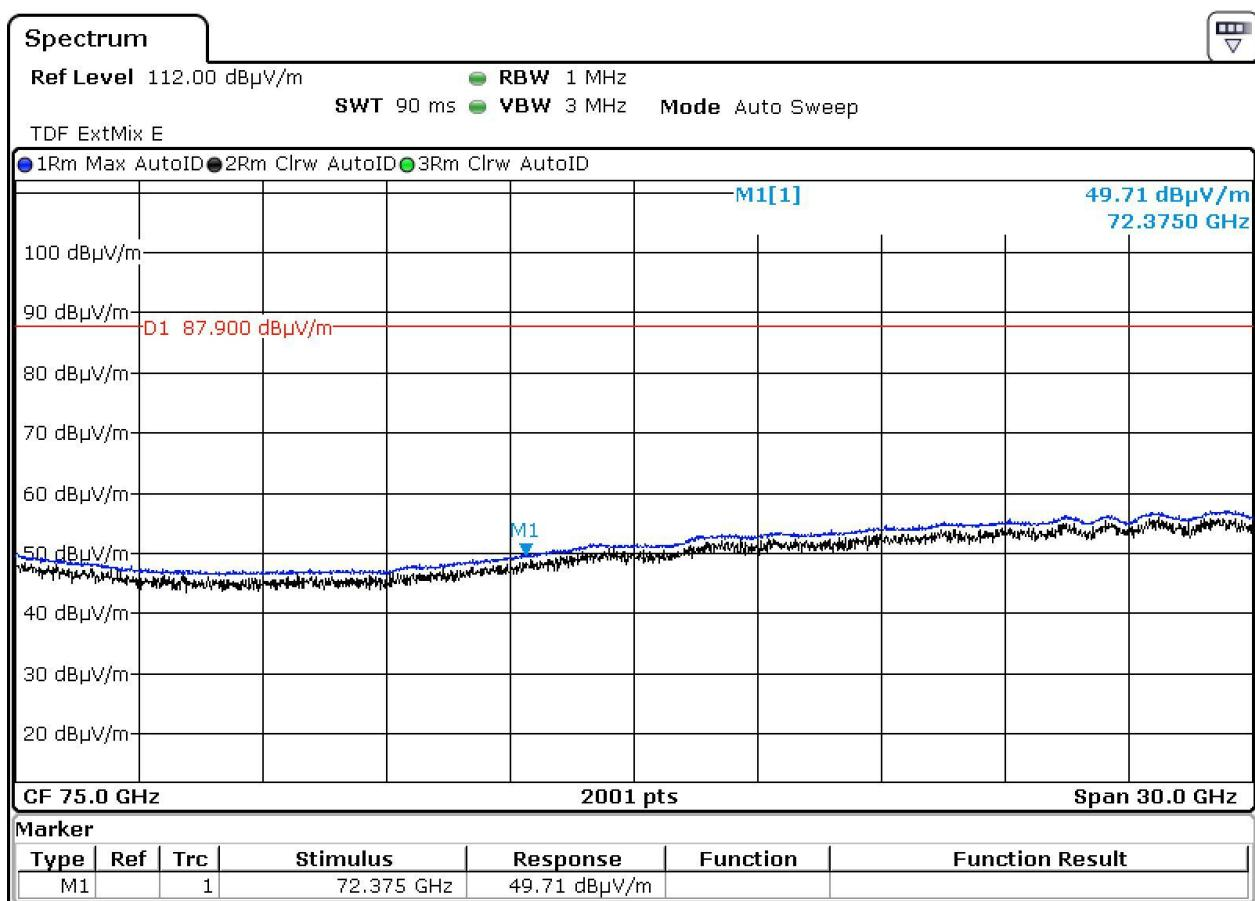
**Test results: Harmonics & Spurious emissions 60 GHz – 90 GHz – Slave Unit**
