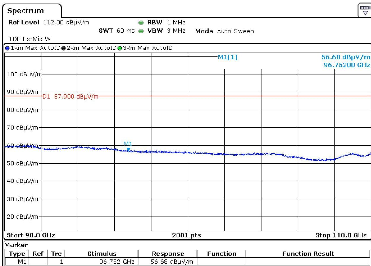
**Test results: Harmonics & Spurious emissions 90 GHz – 110 GHz – Slave Unit**
