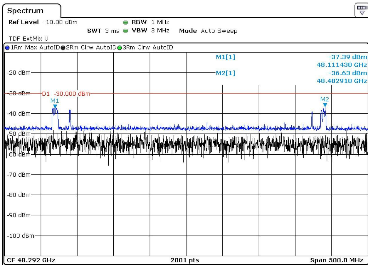
**Test results: Harmonics & Spurious emissions 60 GHz – 90 GHz – Master Unit**
