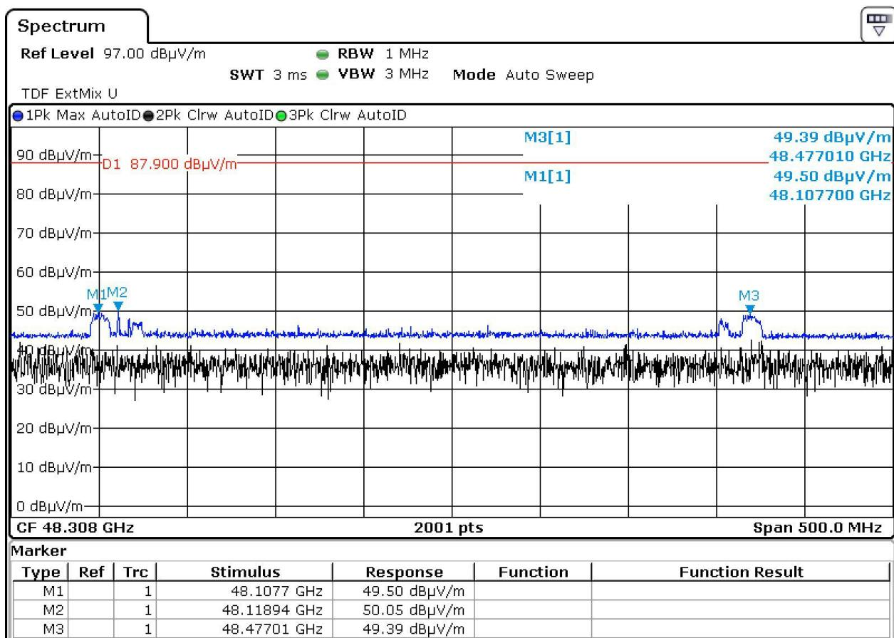
**Test results: Harmonics & Spurious emissions 40 GHz – 60 GHz – Slave Unit**
