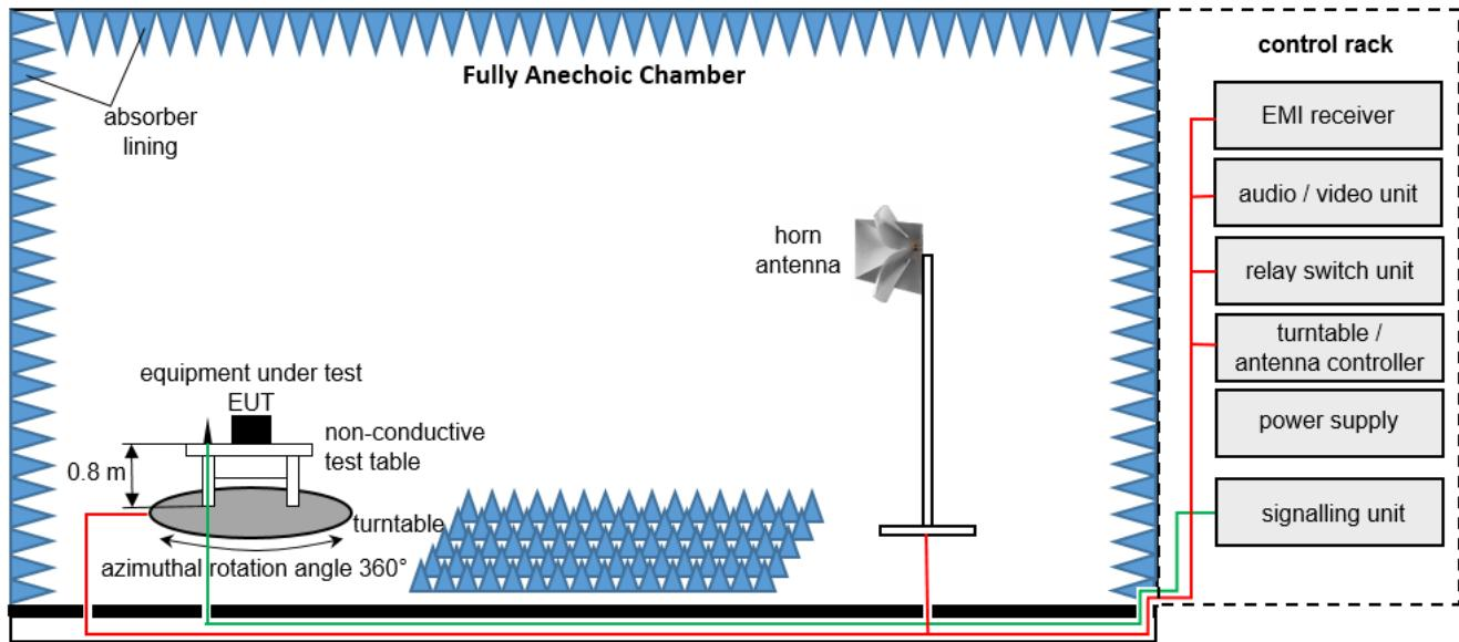
Measurement distance: tri-log antenna and horn antenna 3 meter; loop antenna 3 meter / 1 meter
