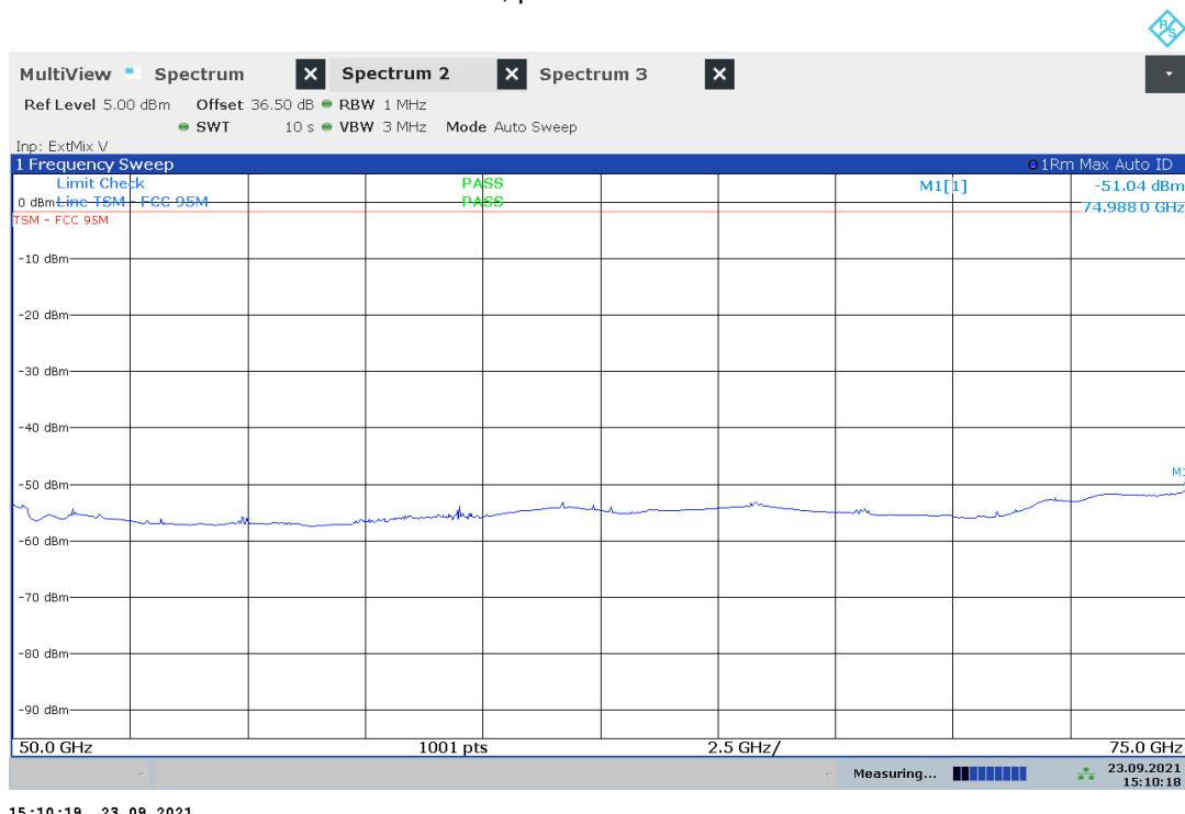
Plot no. 23: radiated emissions 73.5 GHz – 79.5 GHz, BEC, TSM, polarization aligned with radar sensor
