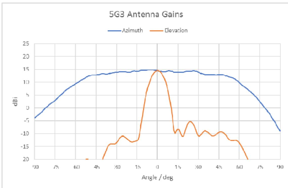
Antenna characteristics in azimuth and in elevation. The peak gain is approx. 15 dBi.
