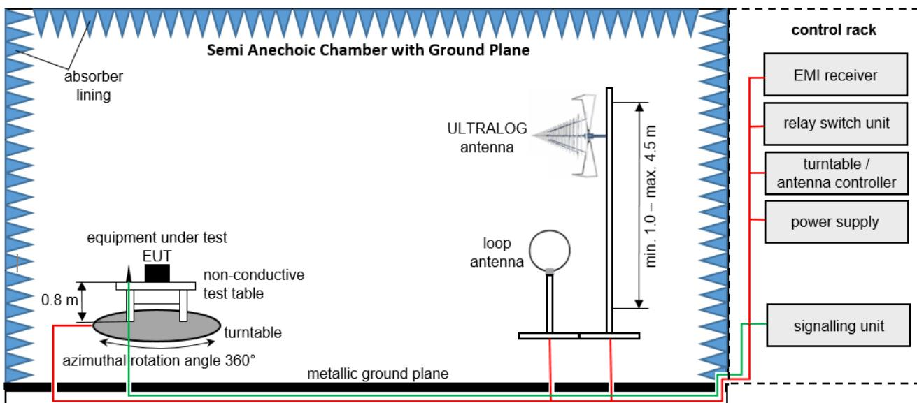
Measurement distance: ULTRALOG antenna 5 meter; loop antenna 5 meter / 3 meter / 1 meter
