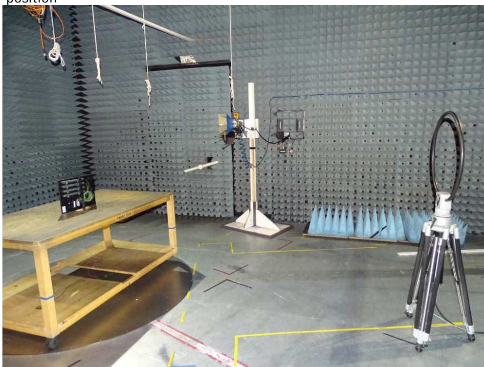
Photo 2: Test setup for radiated emissions measurements in semi-anechoic chamber (9 kHz to 30 MHz), front side view, 3 m measurement distance EUT in horizontal position
