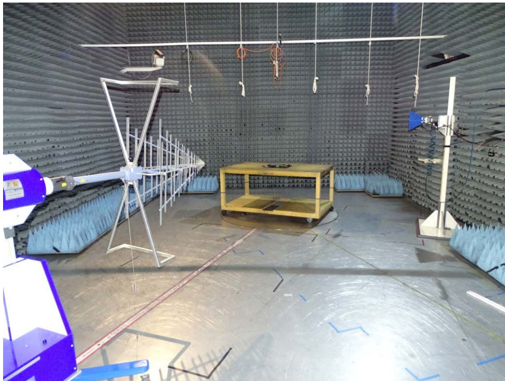
Photo 3: Test setup for radiated emissions measurements in semi-anechoic chamber (30 MHz to 1 GHz), front side view, 3 m measurement distance
