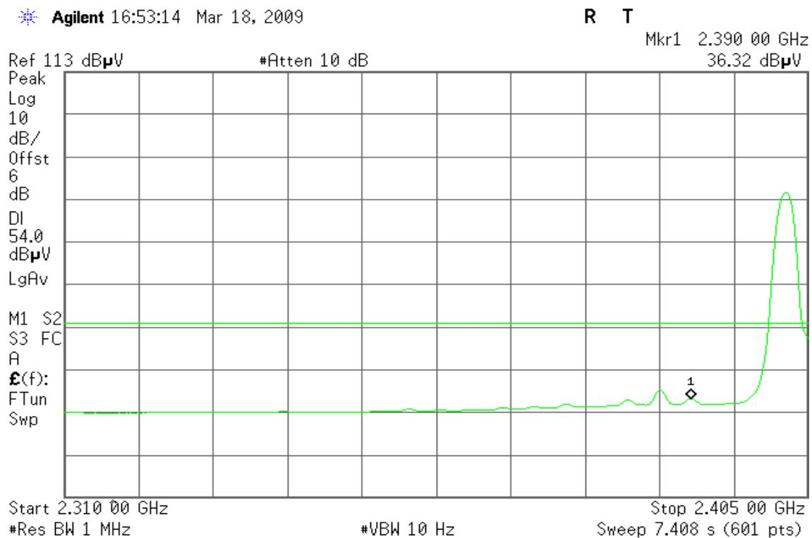
**Band Edges (Bluetooth 8DPSK / CH High)****Detector mode: Peak****Polarity: Vertical**
