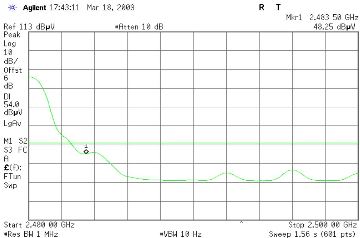
**Band Edges (Bluetooth 8DPSK / CH Low)****Detector mode: Peak****Polarity: Vertical**
