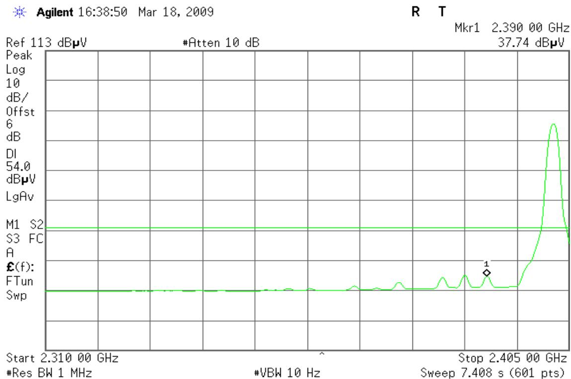
**Band Edges (Bluetooth GFSK / CH High)****Detector mode: Peak****Polarity: Vertical**
