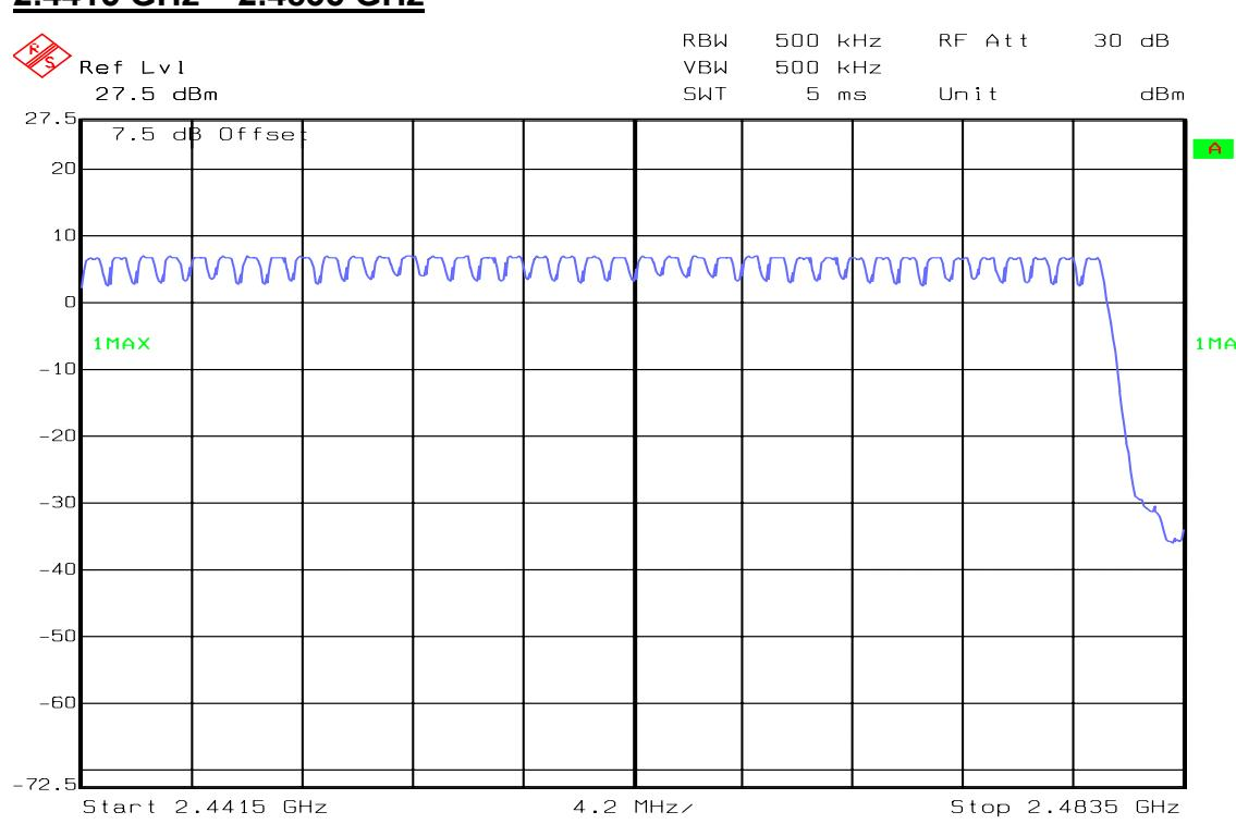
**8DPSK****Channel Number****2.4 GHz – 2.4415 GHz**
