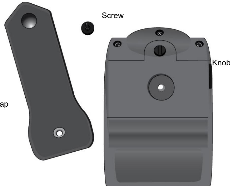
2. Attach the belt strap onto the knob.
