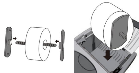
3. Pull a short length of media out of the printer. Close the media cover and press until you hear a click sound to lock it properly:
