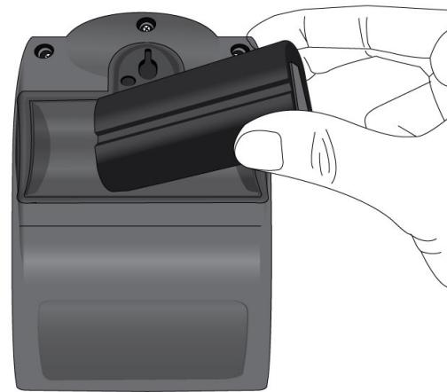
3. Replace the battery cover and turn the battery cover latch 90° to lock in place.
