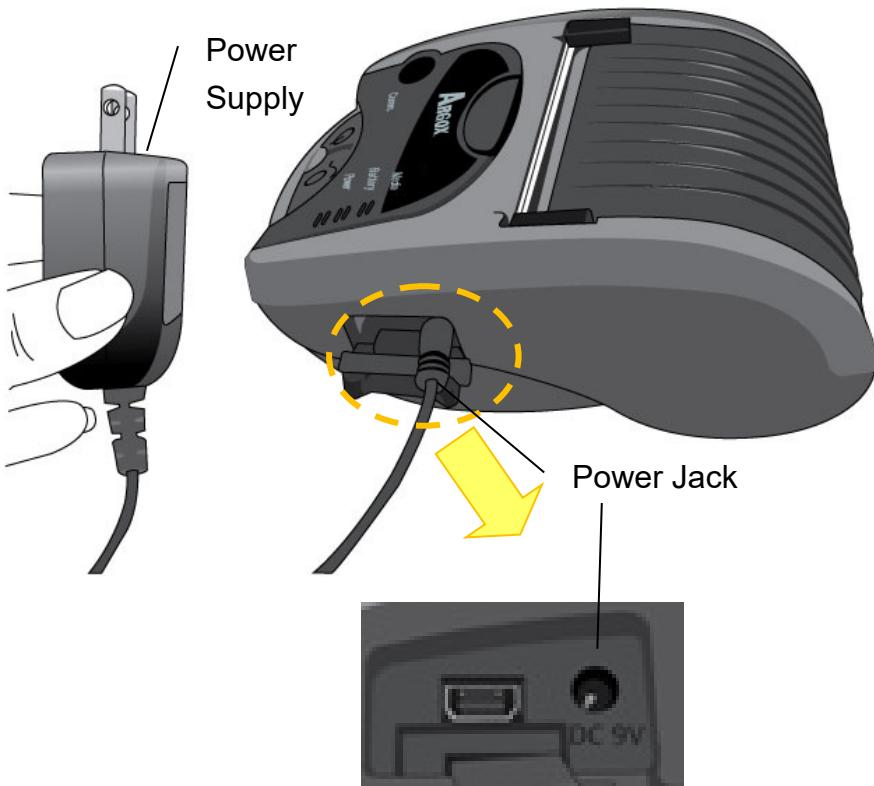
3. The battery is designed for fast charge; after about **3.5 hours (210 minutes)**, the Battery LED will turn off, signifying that the battery is fully charged and ready for use.
