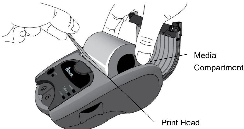
\* If the media supply roll is small, use the media shield to hold the
