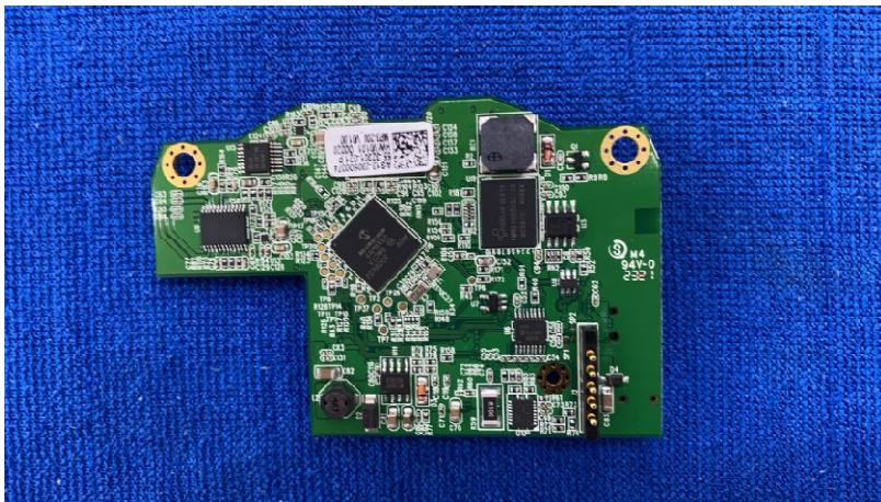
The MP3-200 uses the module and supports Bluetooth 4.2. The IC requires 3.3V for its main power input and the built-in power management unit. A 24MHz XTAL provides the fast clock. An internal PLL is used to generate the 2.4GHz high frequency clock which is output to a bandpass filter and on to the chip antenna. The processor monitors and controls the IC via UART interface with 3.3V level.
