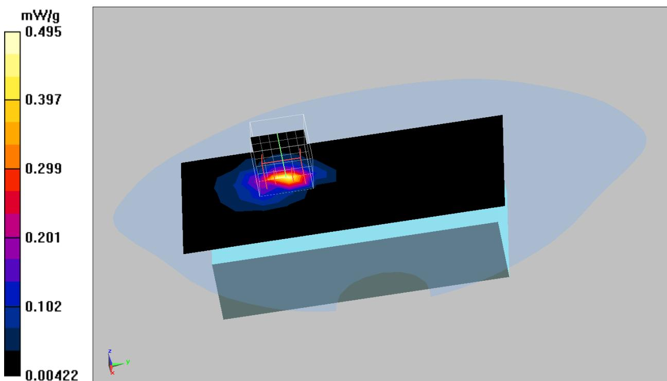
**802.11b EUT Back (GPS Remove) Z-Axis plot****Channel: 11**
