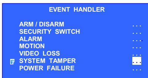
Step 2: Select [SYSTEM TAMPER] option and press “Enter” button to show the system tamper menu and press “Enter” button to enter the System Tamper setting menu.
