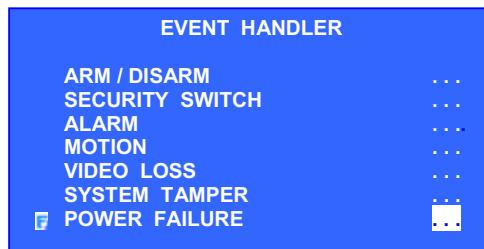
Step 2: Select [POWER FAILURE] option and press “Enter”
