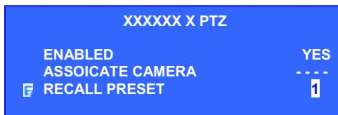
Step 4: Select [RECALL PRESET] option and use the “Left” or “Right” button to select camera and press the “Up” or “Down” button to choose the preset position of the PTZ camera.
