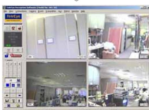
Step 16: Press [**Connect**] icon to connect your PC and the transmitter. The video appears on the WX-30 if success. Otherwise, the **[Warning]** board will pop up and show you failure message. For failure case, please press [**Connect**] icon to check that the connection setting is valid or not.
