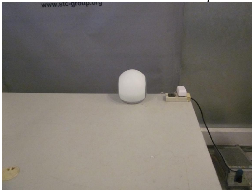
Measurement of Conducted Emission Test Set Up
