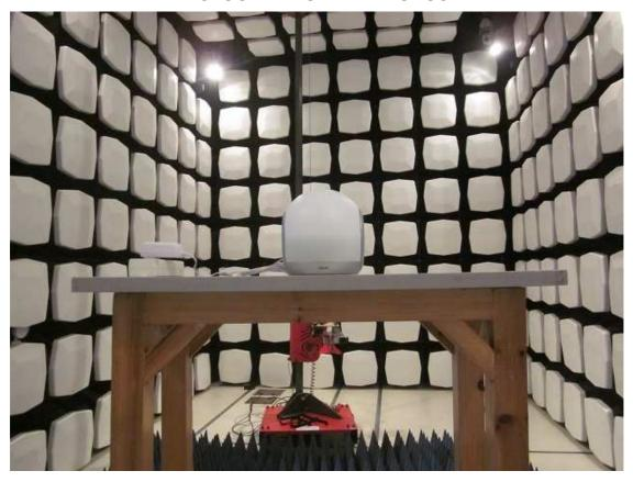
**MEASUREMENT OF CONDUCTED EMISSION TEST SET UP**
