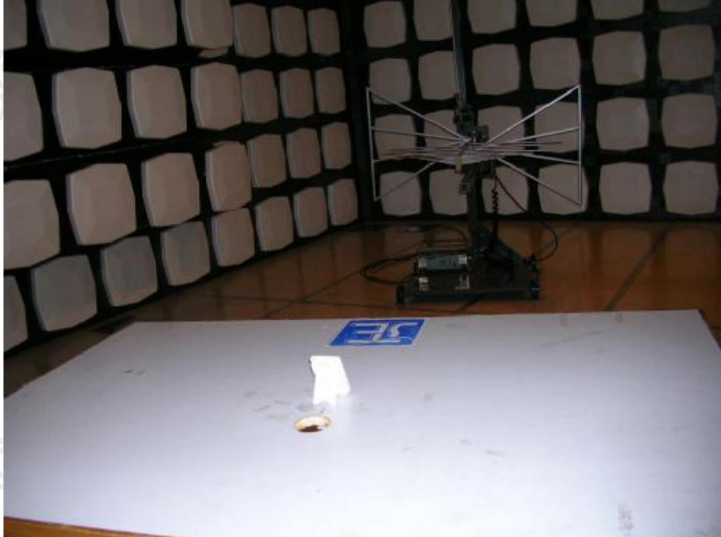
Measurement of Radiated Emission Test Set Up
