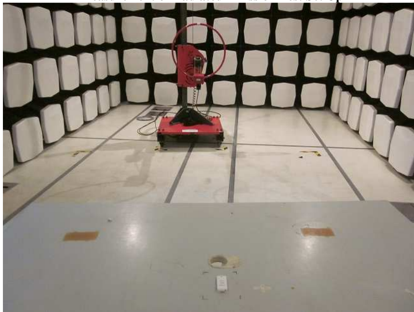
Measurement of Radiated Emission Test Set Up
