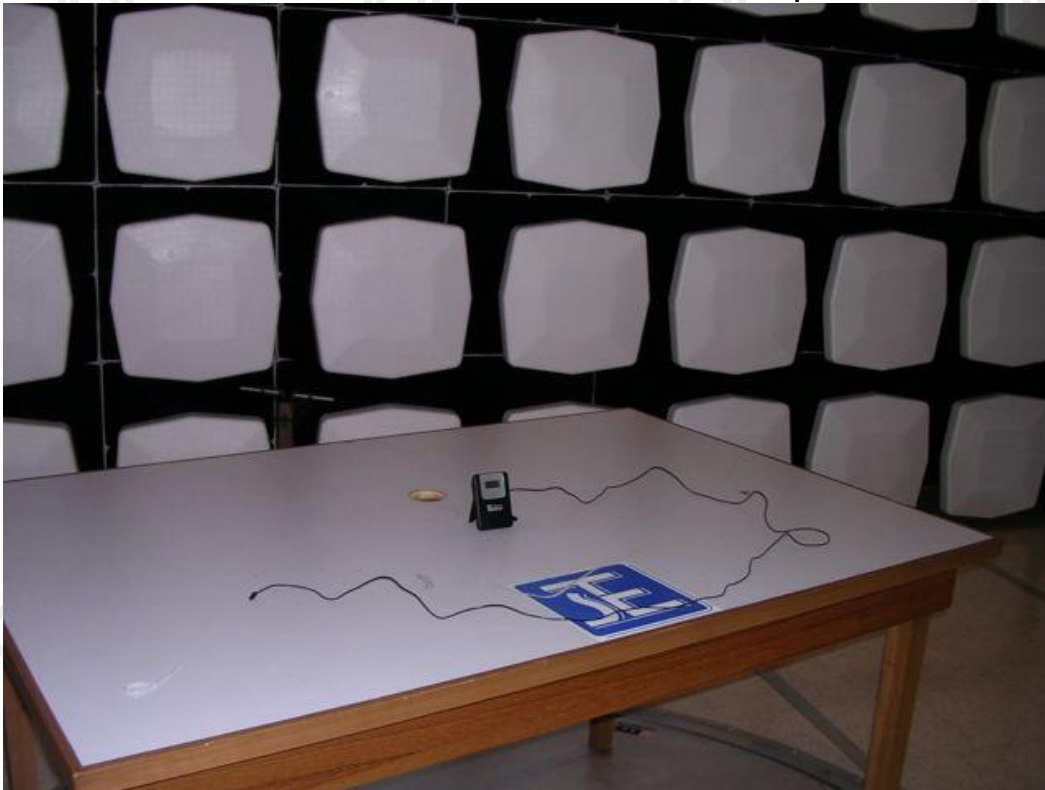
Measurement of Radiated Emission Test Set Up
