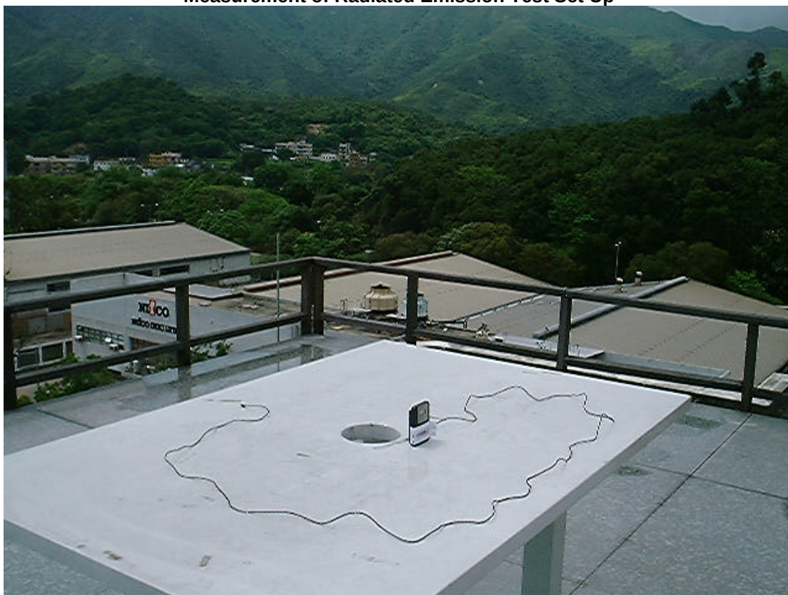
Measurement of Radiated Emission Test Set Up
