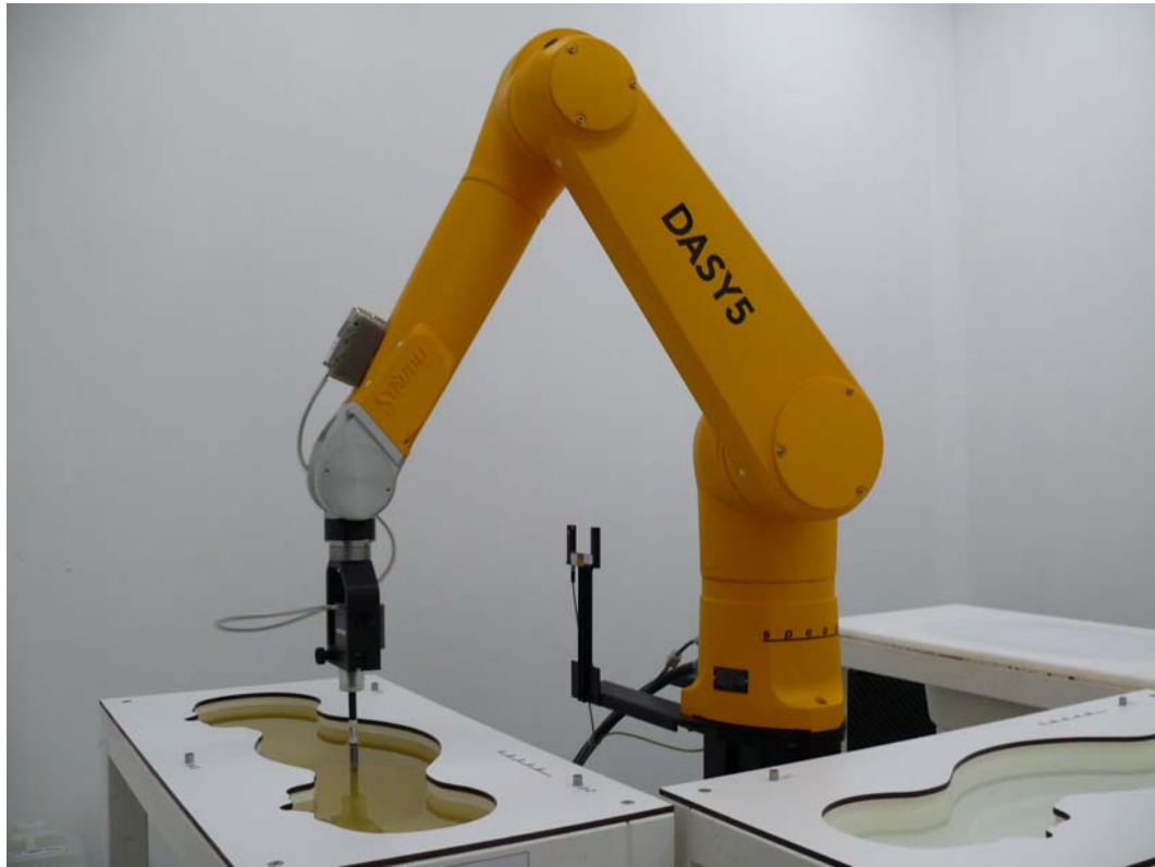
Picture 1: Specific Absorption Rate Test Layout
