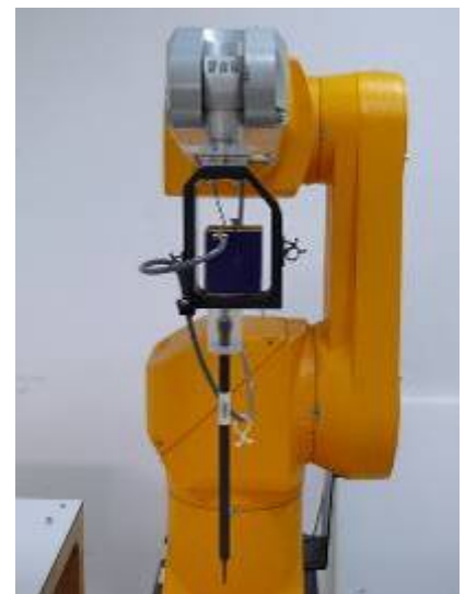
Figure 3. EX3DV4 E-field probe
