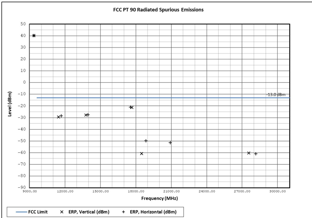
**Note:** All recorded data was plotted. Six (6) or more of the highest emissions of the worst-case operational mode of the EUT are represented below in tabular format. Emissions 20 dB below the limit are not required to be reported.
