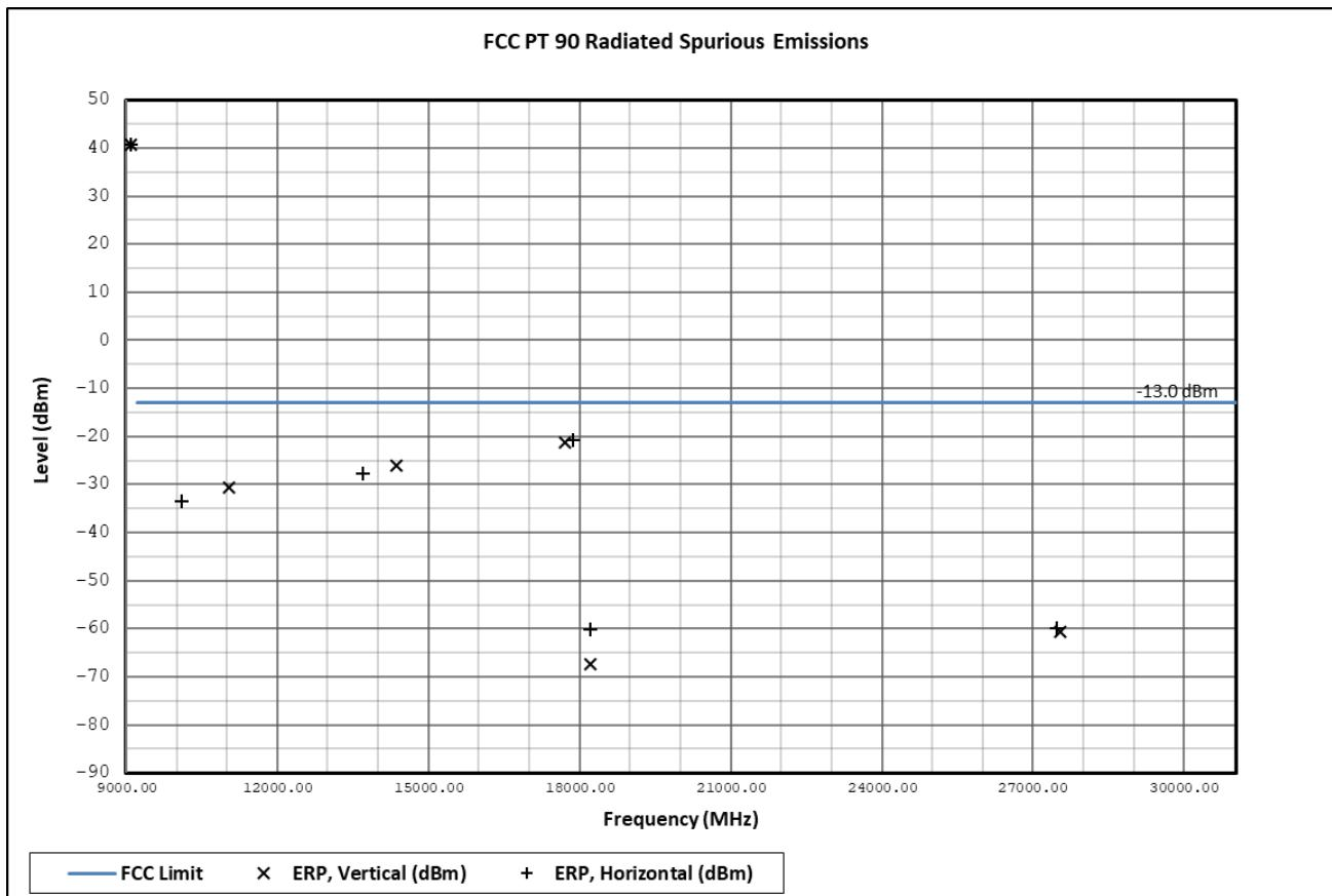
**Note:** All recorded data was plotted. Six (6) or more of the highest emissions of the worst-case operational mode of the EUT are represented below in tabular format. Emissions 20 dB below the limit are not required to be reported.
