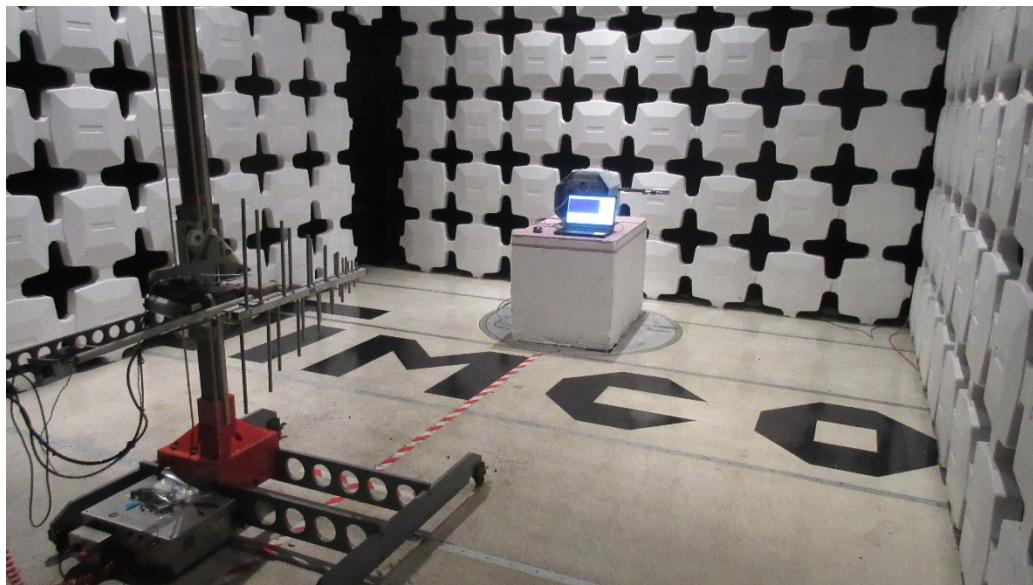
Radiated Testing, Above 1 GHz
