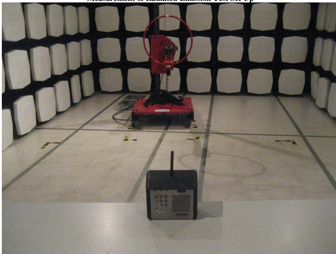
Measurement of Radiated Emission Test Set Up
