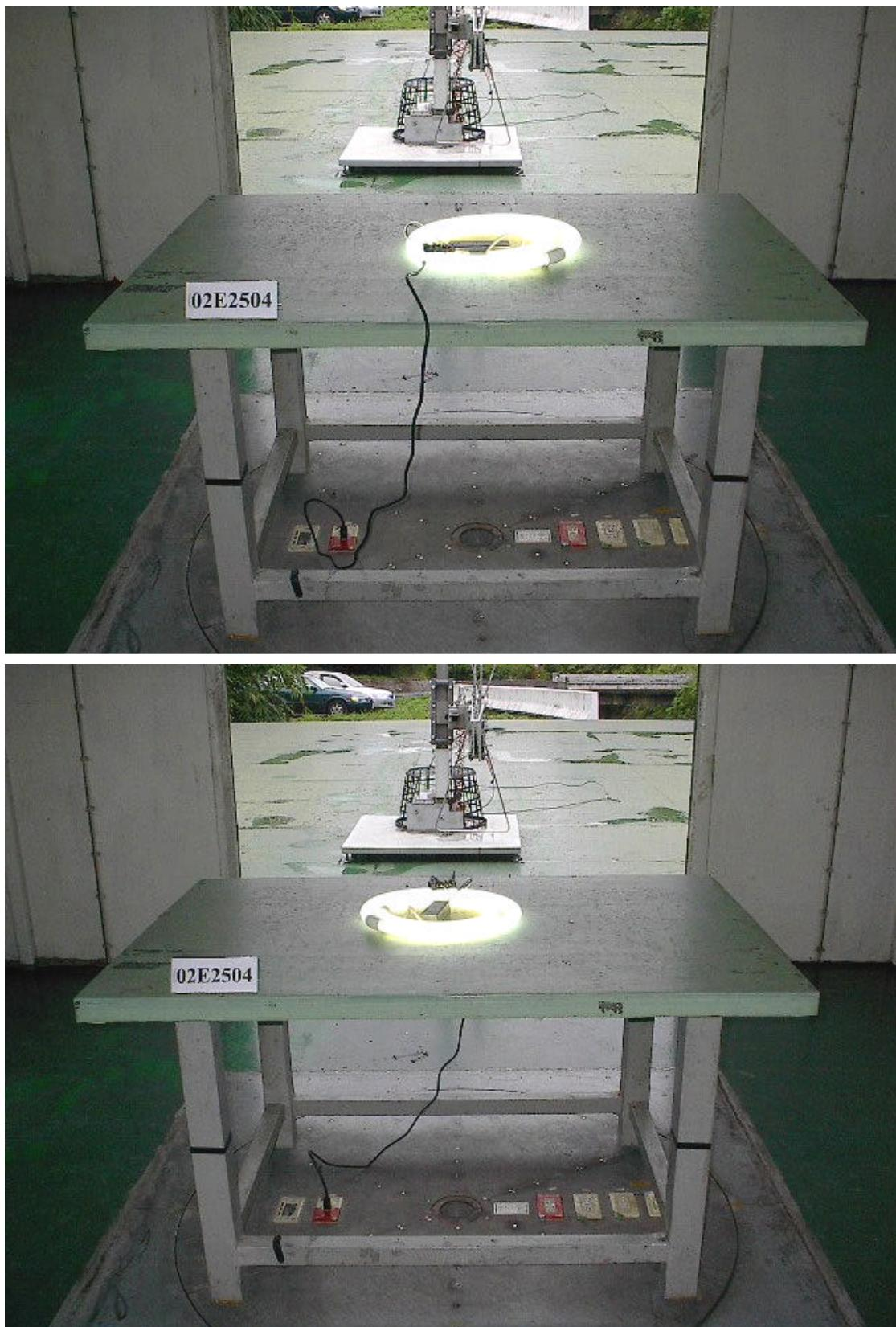
**5-2. Radiated Measurement Photos      Test Mode : Loop Antenna**
