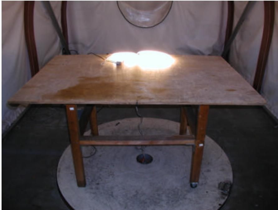
**6.16 FC8T9 22W + FC12T9 32W Conducted Emission Photograph – Rear View**
