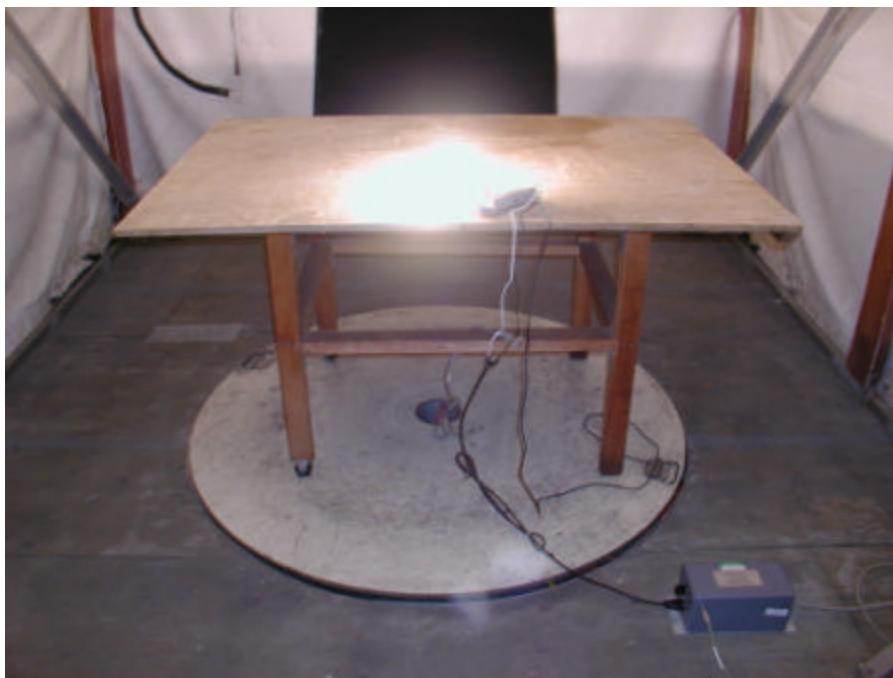
**6.15 FC8T9 22W + FC12T9 32W Conducted Emission Photograph – Front View,**
