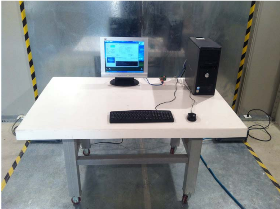
Conducted Emissions - Side View
