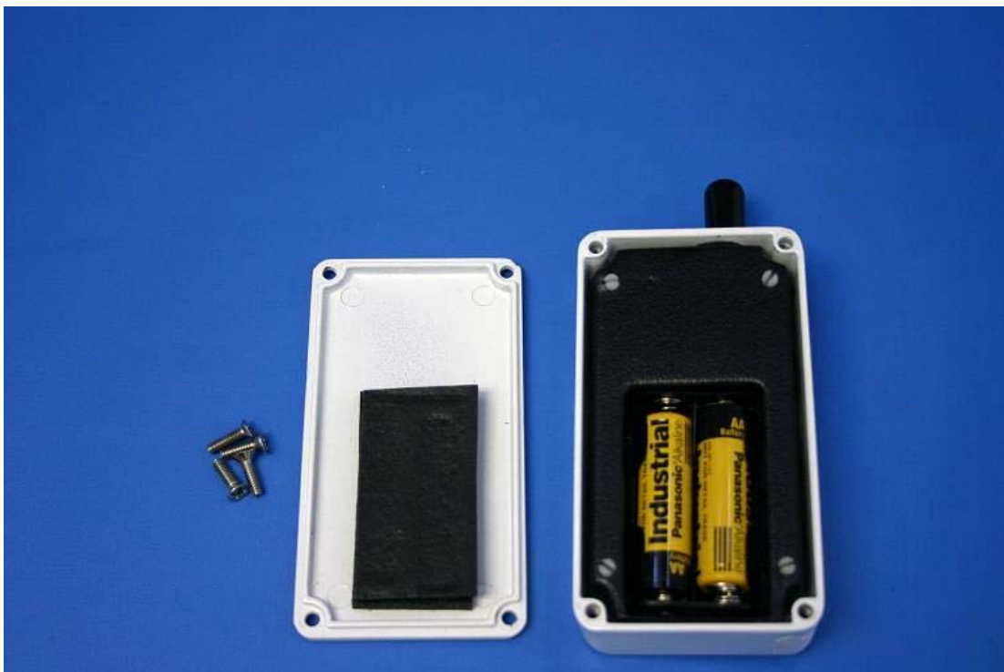
Figure 2: Eight Channel Transmitter with Back Plate Removed
