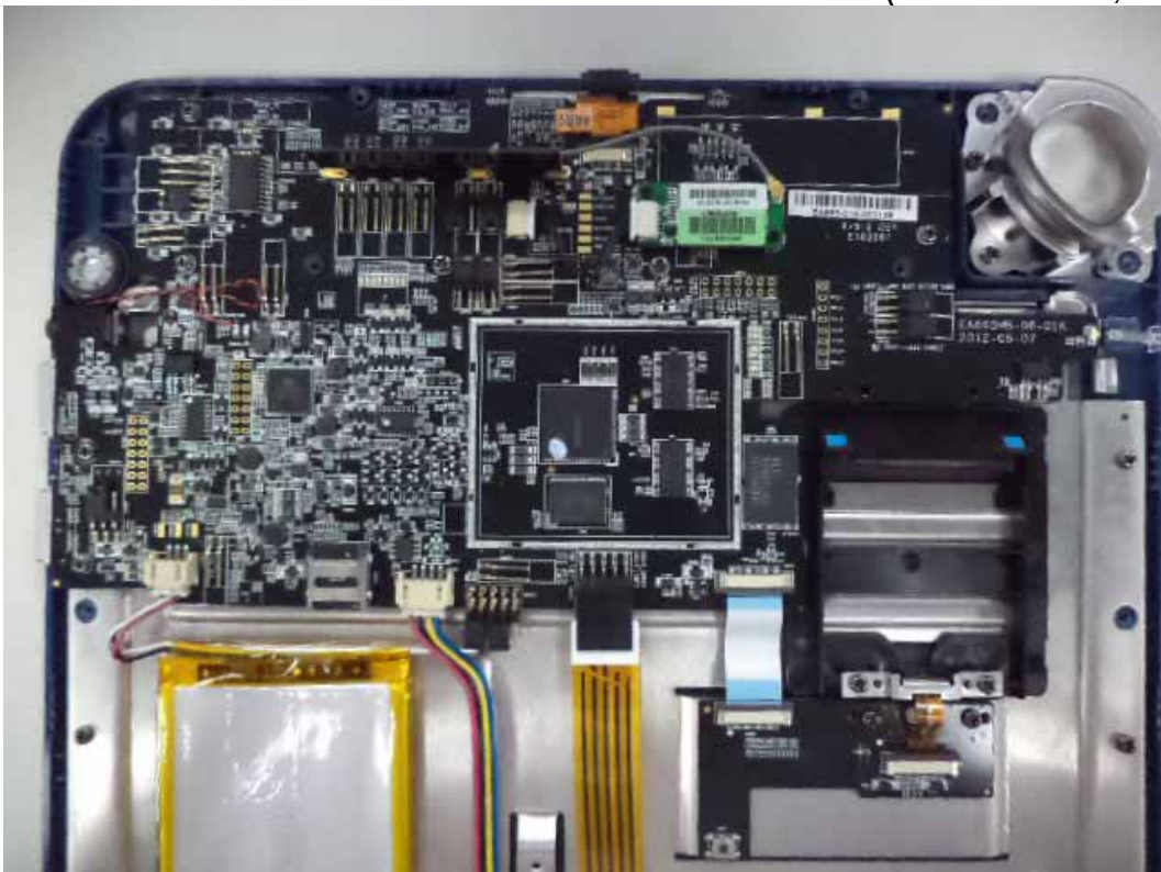
Figure 4 Internal View (Control Board, Front View)
