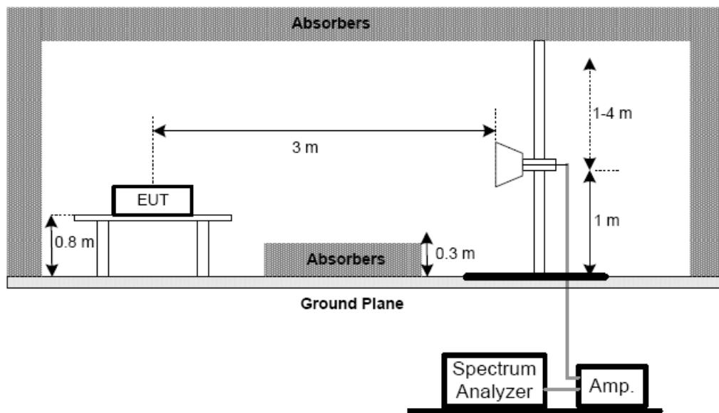
(C) For radiated emissions below 30MHz
