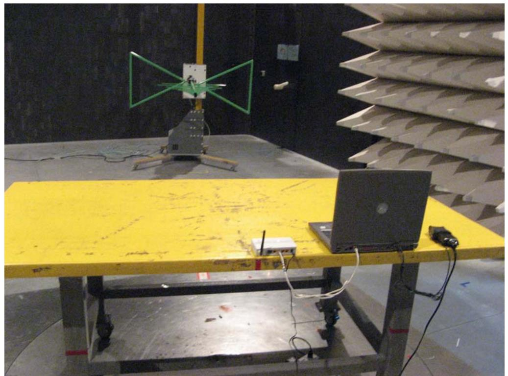
**For radiated emissions above 1GHz****FRONT VIEW**
