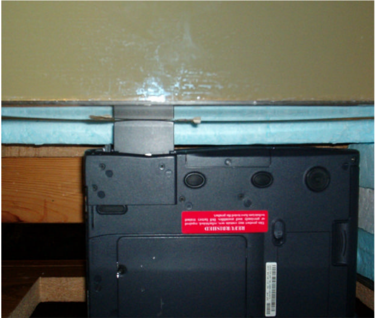
Fig. 3. Photograph of the Dell Model PP01L Host Computer at 90° with the edge of the Cybertan Technology Wireless LAN Cardbus Card Model WE701-I pressed against the bottom of the planar phantom. This is Configuration 2 for SAR testing and represents the case of a bystander at a distance of 0 cm from the edge of the Cardbus Card.
