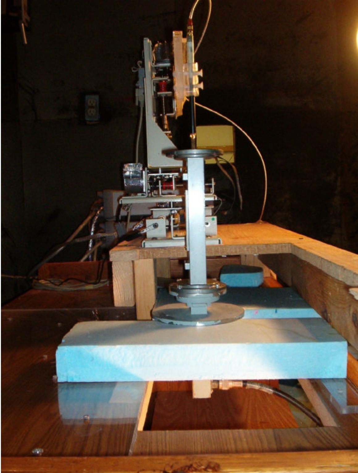
Fig. 6b. Photograph of the waveguide setup showing also the coax to waveguide coupler at the bottom used to feed power to the vertical waveguide containing the tissue-simulant fluid.
