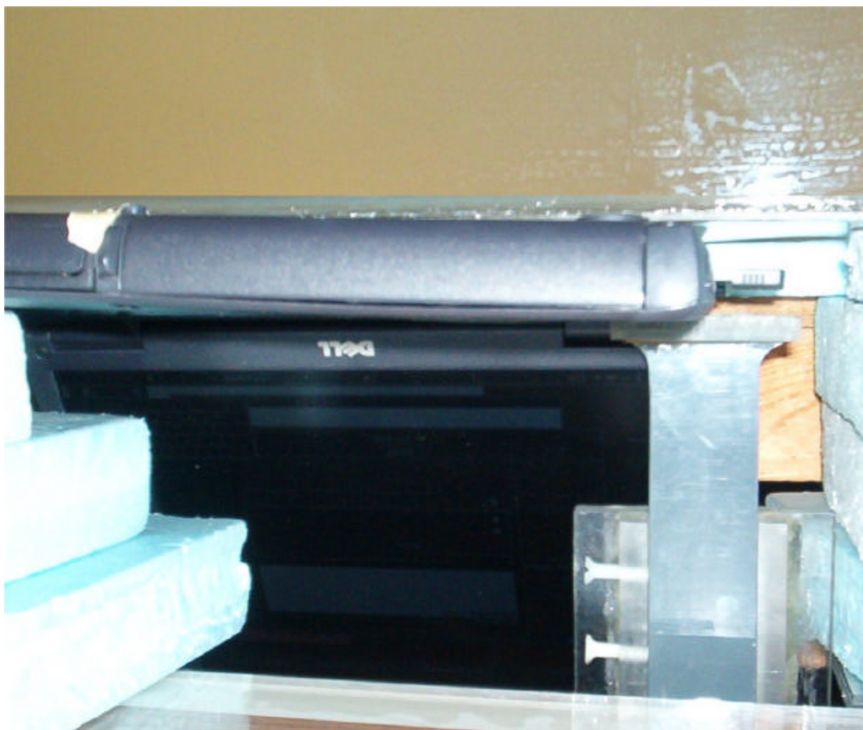
Fig. 2. Photograph of the bottom of the Dell Model PP01L Host Computer with Cybertan Technology Wireless LAN Cardbus Card Model WE701-I pressed against the bottom of the planar phantom. This Configuration 1 – Laptop position for SAR testing.
