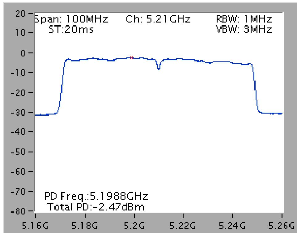
Power Density Plot on Configuration IEEE 802.11a / Ant. 1 + Ant. 2 + Ant. 3 / 5240 MHz
