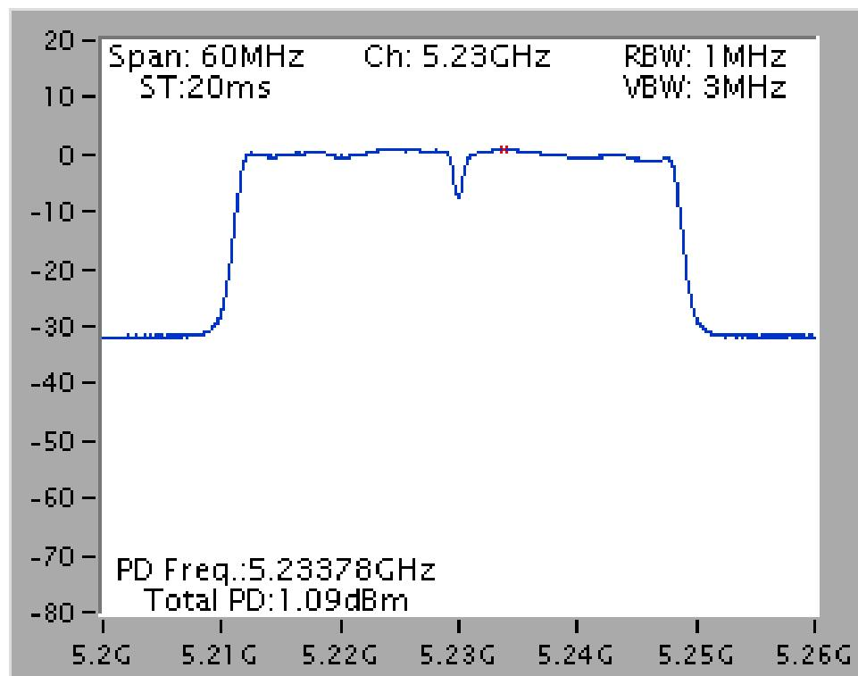
Power Density Plot on Configuration IEEE 802.11ac MCS0 VHT 80MHz / Ant. 1 + Ant. 2 + Ant. 3 / 5210 MHz
