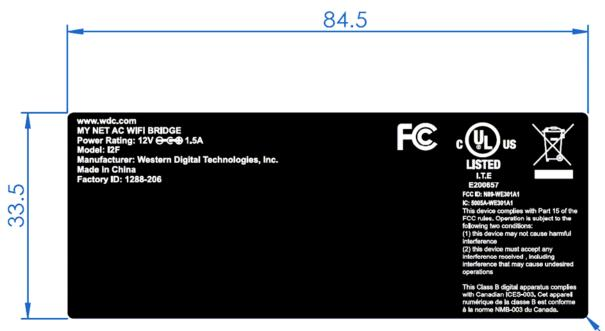
SIZE: 84.5x33.5mm(tolerance +/-0.2mm),R1.0mmx4
