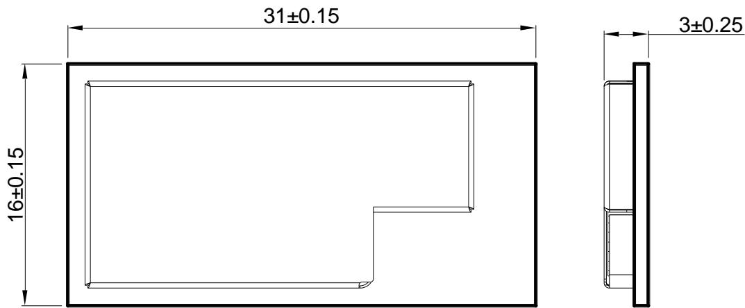
**Figure 1: PCB Outline Top View (Unit: mm)**
