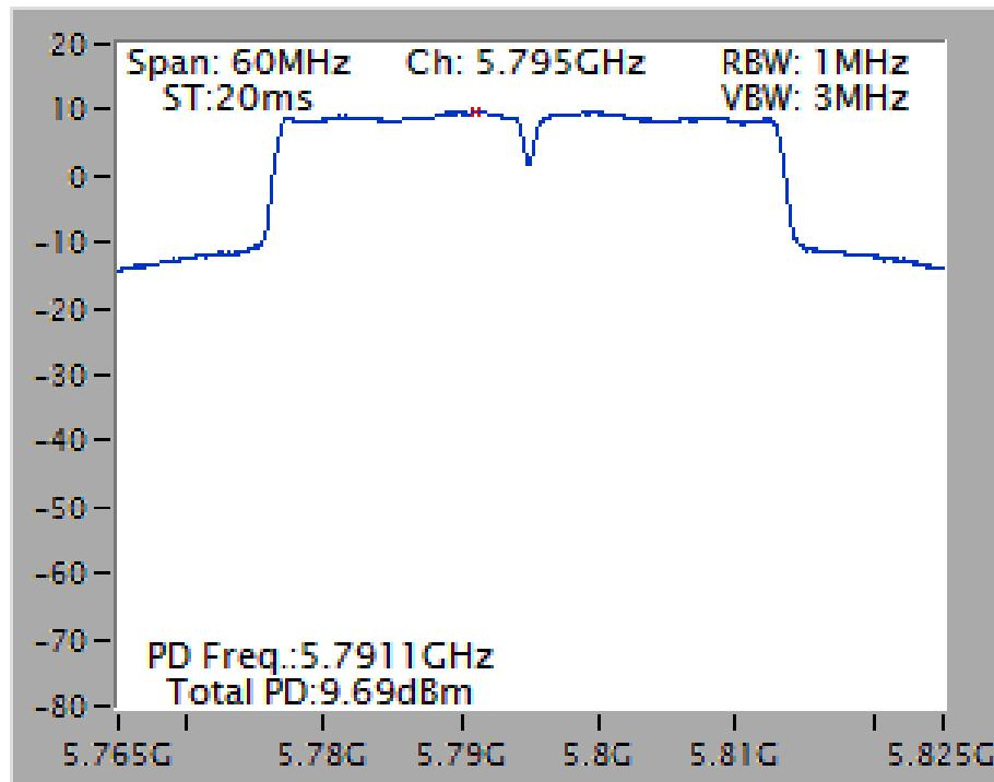
**Power Density Plot on Configuration IEEE 802.11ac MCS0/Nss1 VHT80 / Ant. 3 + Ant. 4 + Ant. 5 / 5775 MHz**
