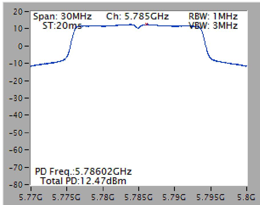
**Power Density Plot on Configuration IEEE 802.11ac MCS0/Nss1 VHT40 / Ant. 3 + Ant. 4 + Ant. 5 / 5795 MHz**
