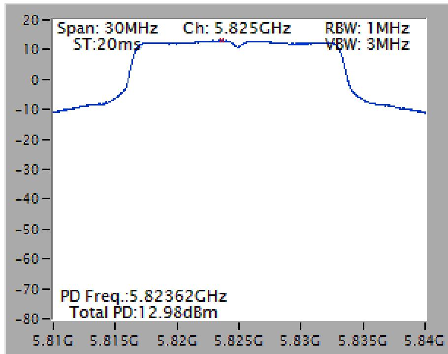
Power Density Plot on Configuration IEEE 802.11ac MCS0/Nss1 VHT20 / Ant. 3 + Ant. 4 + Ant. 5 / 5785 MHz
