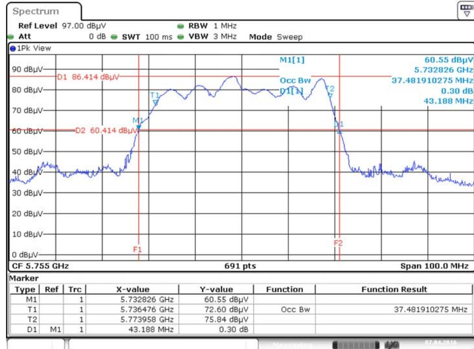
**26dB Bandwidth and 99% Occupied Bandwidth Plot on Configuration IEEE 802.11n MCS0 HT40 / Ant. 1 + Ant. 2 + Ant. 3 + Ant. 4 / 5795 MHz**
