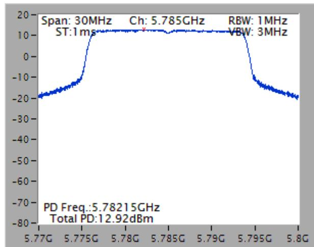
**Power Density Plot on Configuration IEEE 802.11n MCS0 HT40 / Ant. 1 + Ant. 2 + Ant. 3 + Ant. 4 / 5795 MHz**
