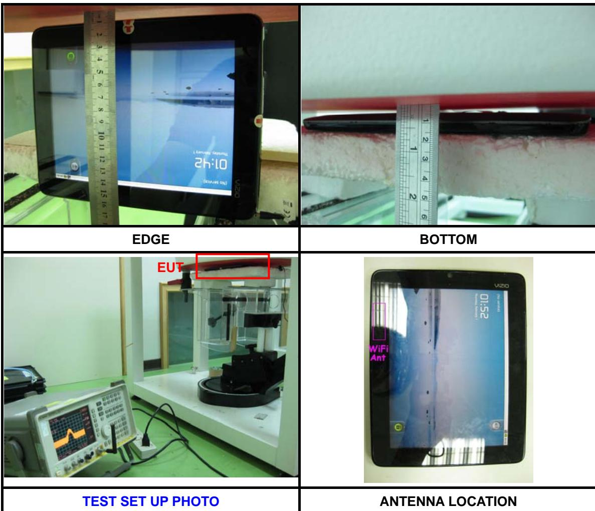
**NOTE:** The EUT face to the phantom with 5mm-separation distance.
