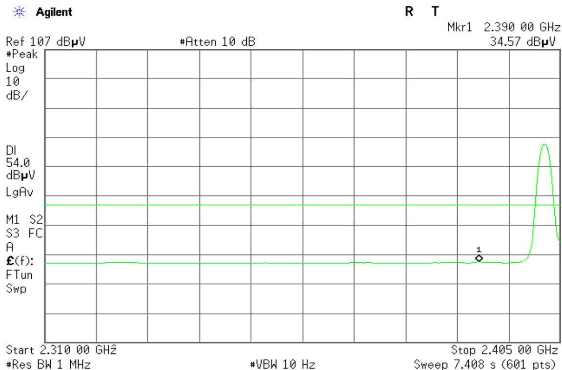
**Band Edges (CH High)****Detector mode: Peak****Polarity: Vertical**
