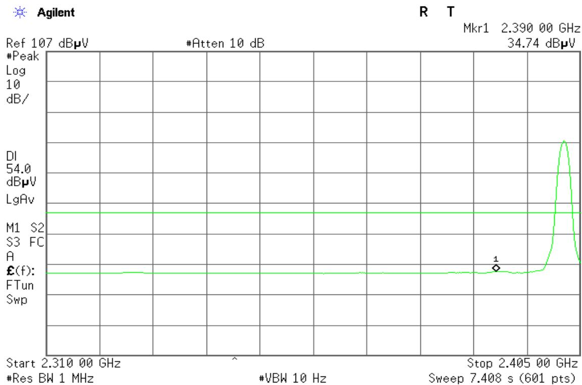
**Band Edges (CH High)****Detector mode: Peak****Polarity: Vertical**
