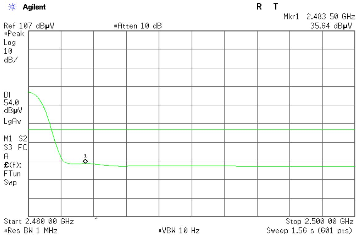
**Detector mode: Peak****Polarity: Horizontal**
