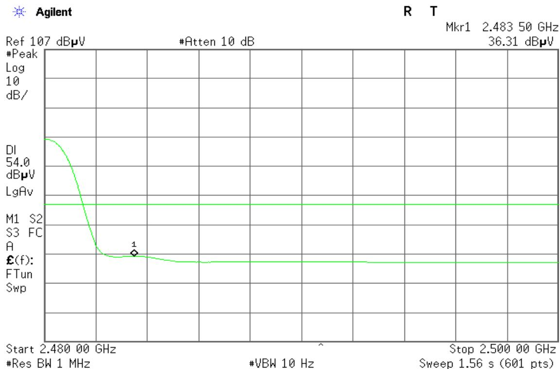
**For 8DPSK / DH5****Band Edges (CH Low)****Detector mode: Peak****Polarity: Vertical**
