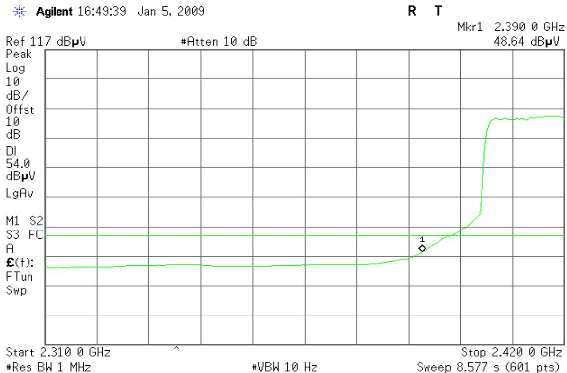
**Band Edges (IEEE 802.11g / CH High)****Detector mode: Peak****Polarity: Vertical**
