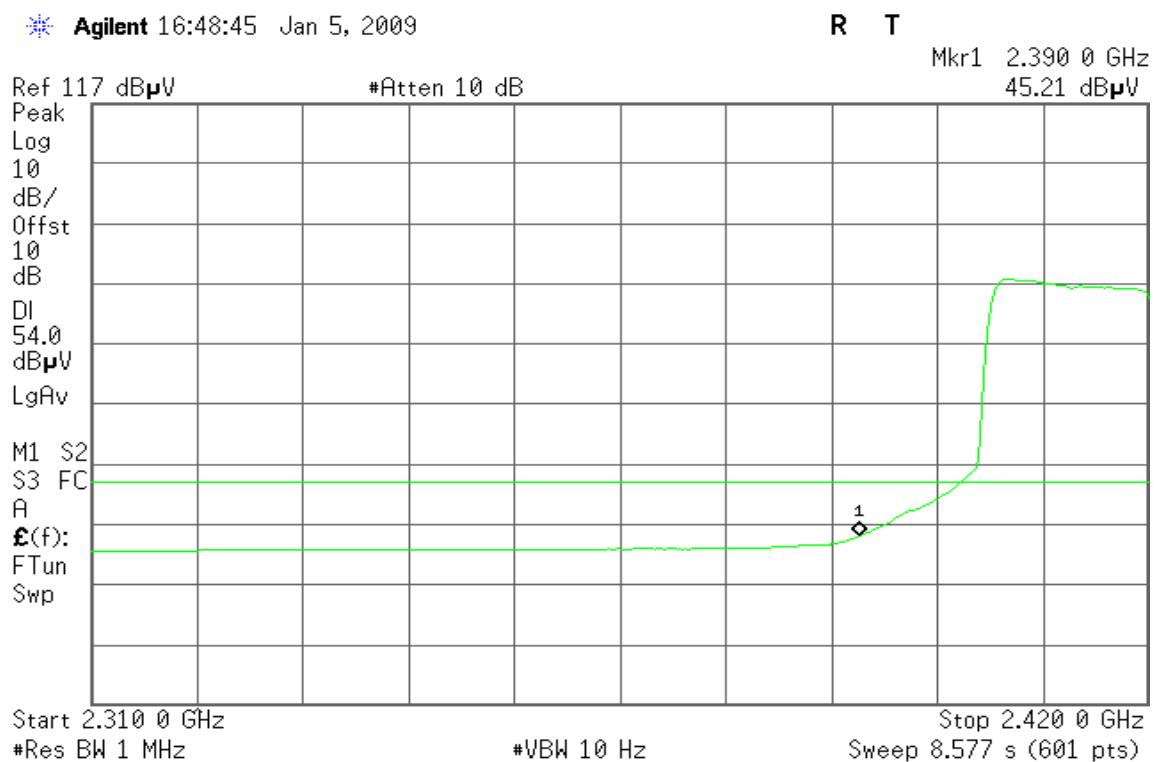
**Detector mode: Peak****Polarity: Horizontal**
