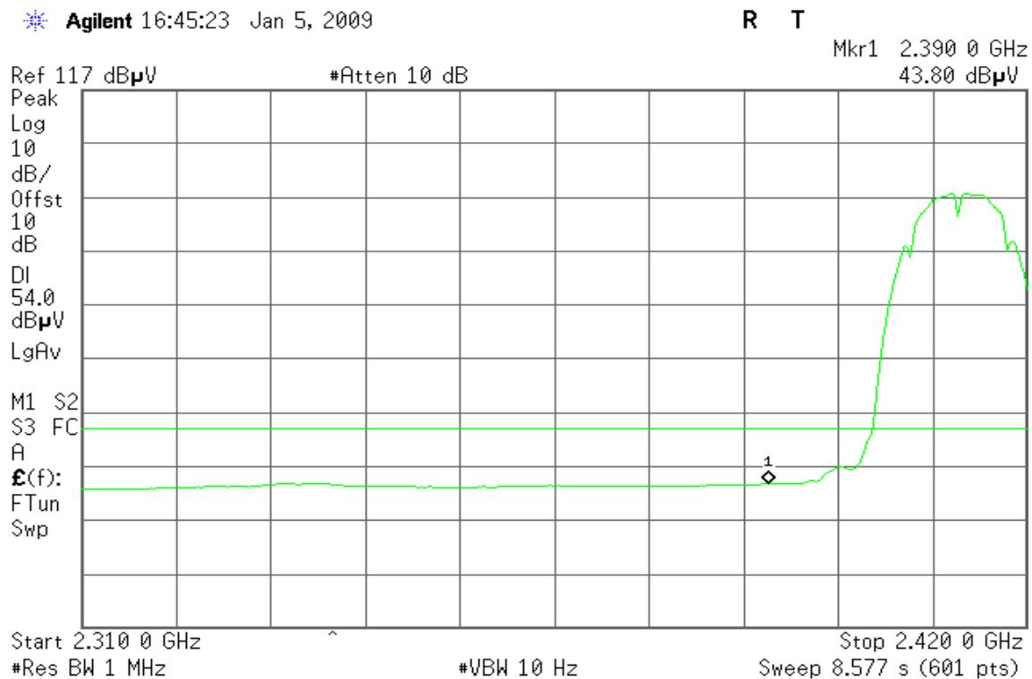
**Band Edges (IEEE 802.11b / CH High)****Detector mode: Peak****Polarity: Vertical**
