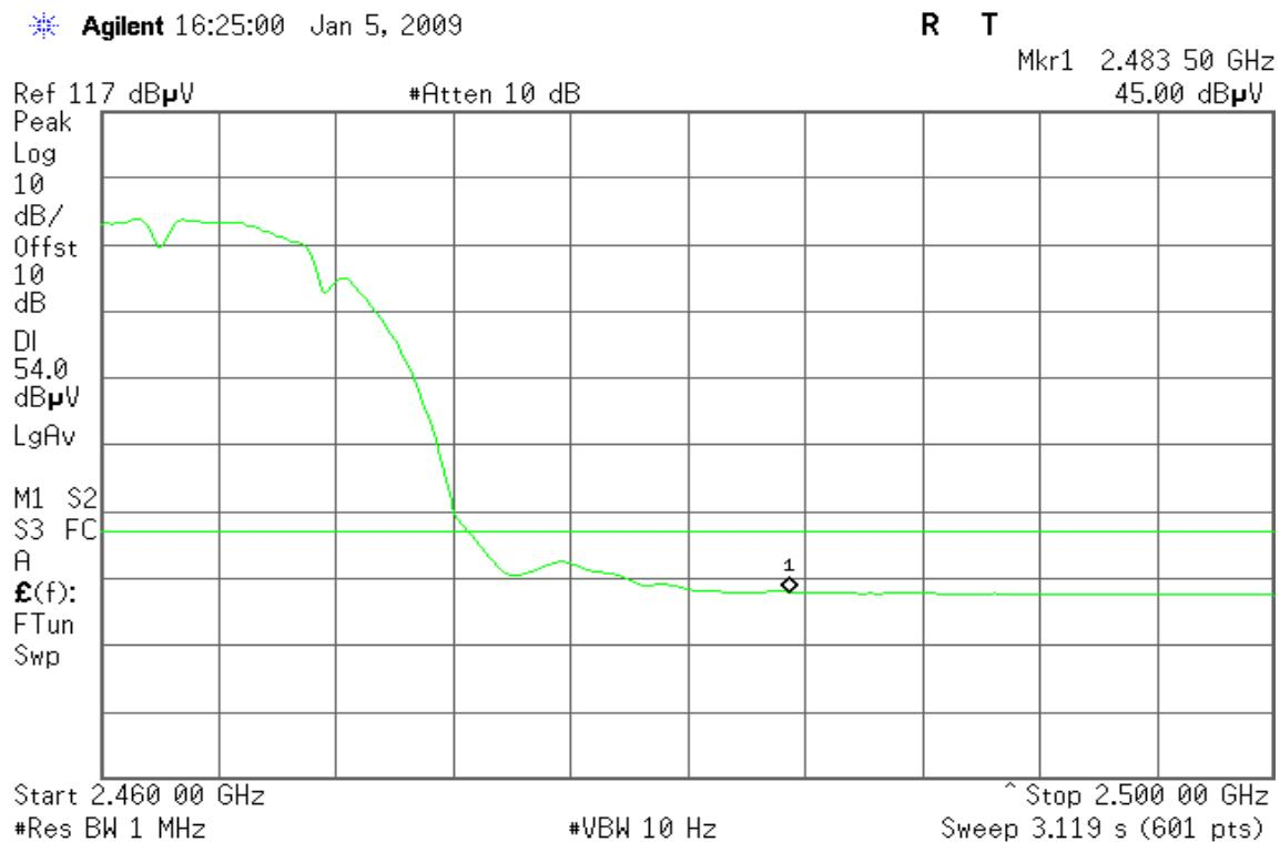
**Band Edges (IEEE 802.11g / CH Low)****Detector mode: Peak****Polarity: Vertical**
