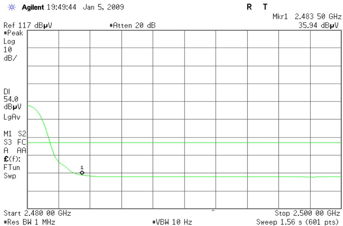
**For 8DPSK / DH5****Band Edges (CH Low)****Detector mode: Peak****Polarity: Vertical**
