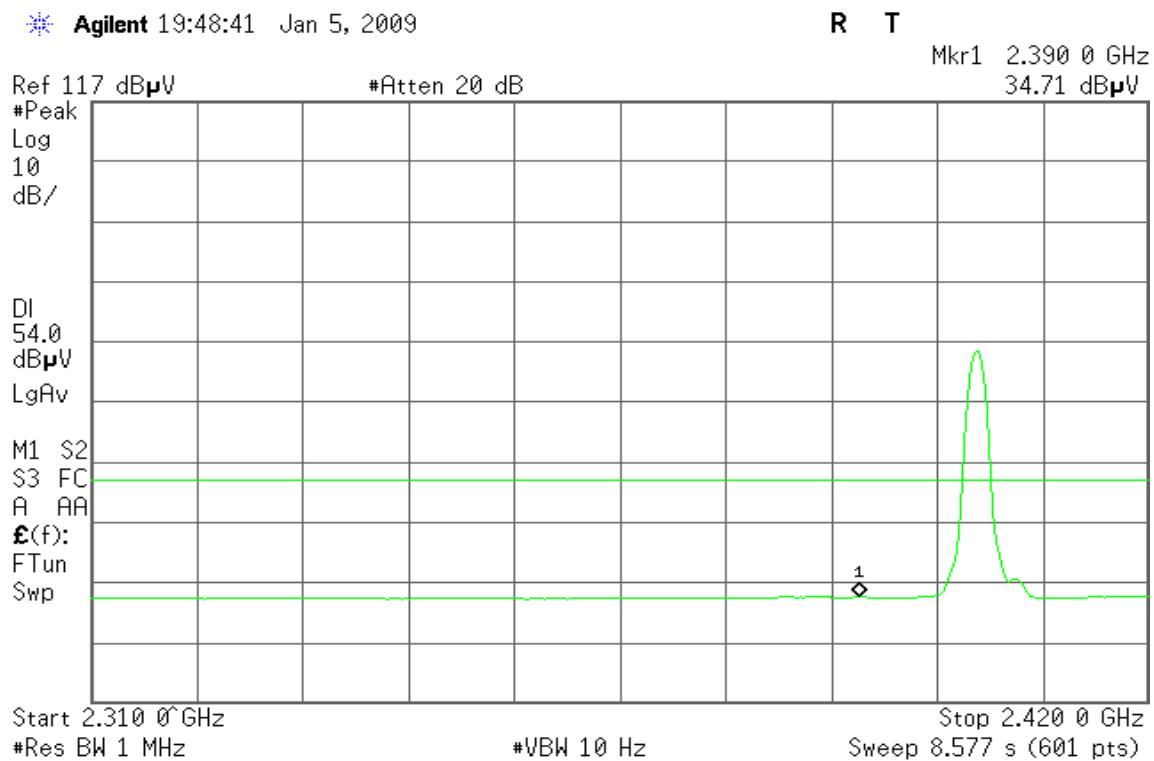
**Band Edges (CH High)****Detector mode: Peak****Polarity: Vertical**
