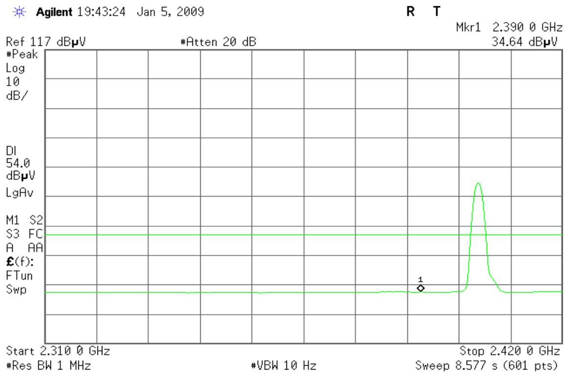
**Band Edges (CH High)****Detector mode: Peak****Polarity: Vertical**
