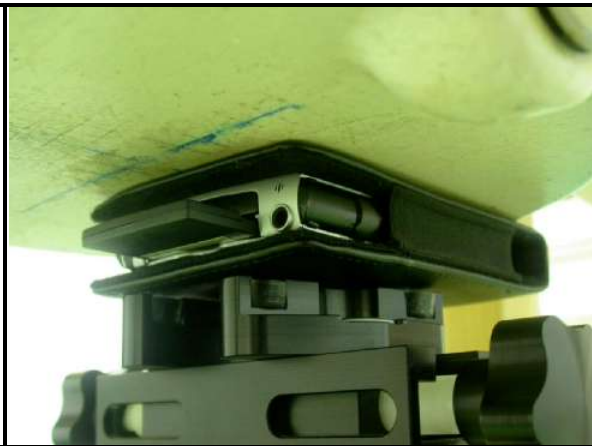
B: The front of the EUT face to the phantom with 14mm-separation distance.
