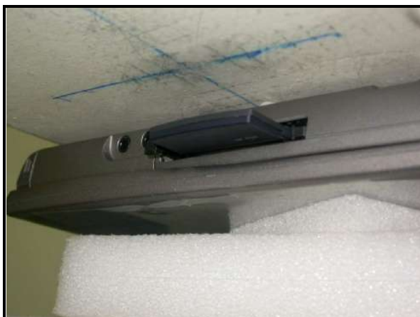
C: The bottom of the EUT face to the phantom with 17mm-separation distance.
