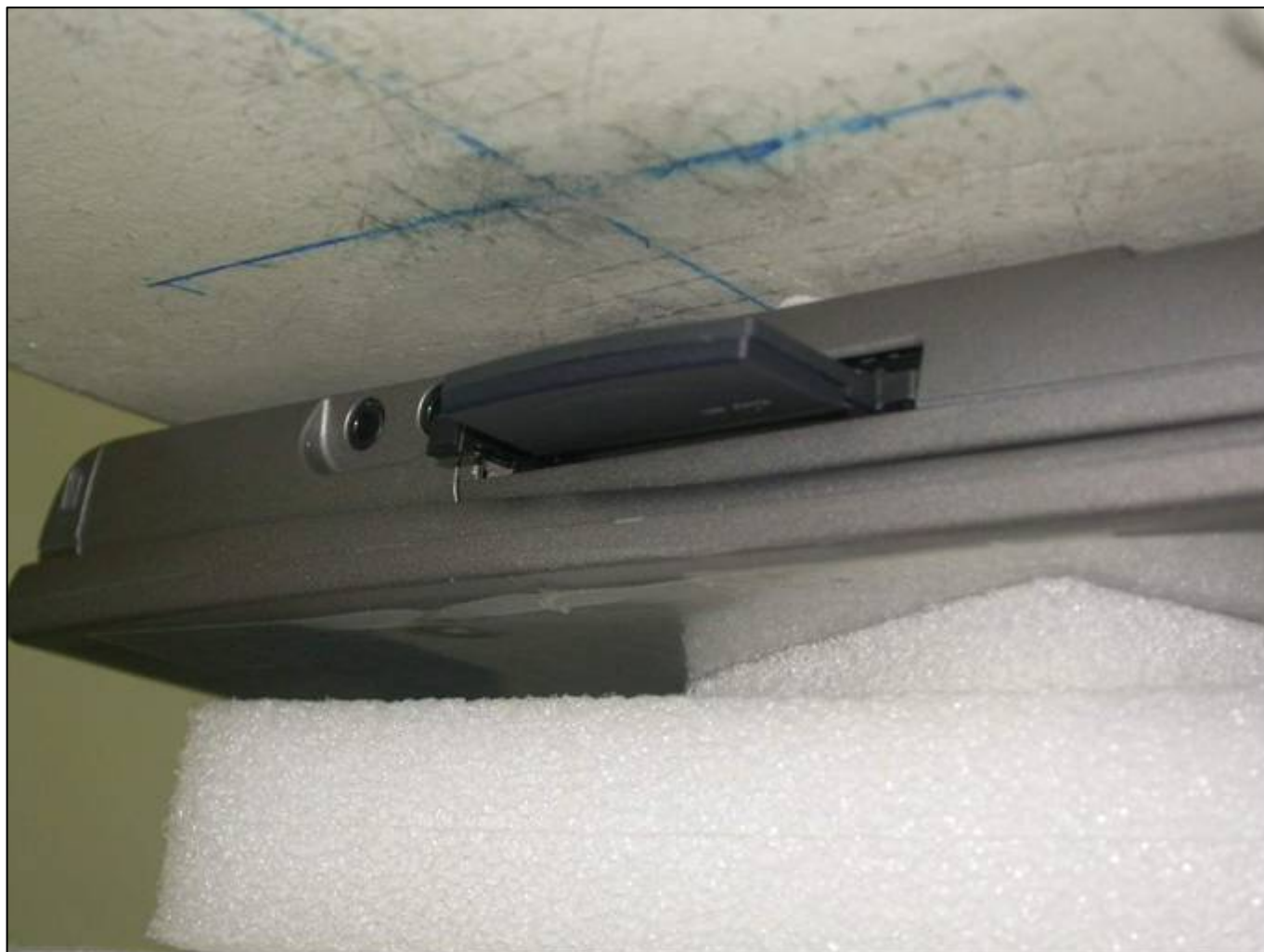
The Bottom of the EUT to the flat phantom distance 17 mm
